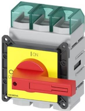
SENTRON, Switch disconnector 3LD, emergency switching-off switch, 3-pole,  $I_{lu}$ : 160 A, operating power / at AC-23 A 400 V: 75 kW, front-mounted, knob-operated mechanism, red/yellow, 4-hole mounting of the handle
