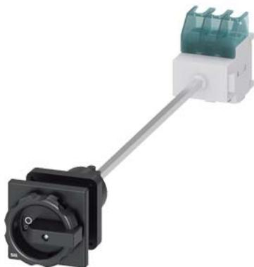
SENTRON, Switch disconnector 3LD, main switch, 3-pole,  $I_u$ : 25 A, Operating power / at AC-23 A at 400 V: 9.5 kW, floor mounting with door coupling, rotary operating mechanism, black, central mounting 22.5 mm of the handle
