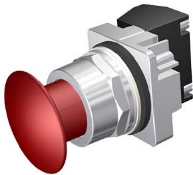
30mm Command/52, Chrome Finish Heavy Duty, Watertight/Oiltight Complete Metal Unit Push-Pull Operator Non-Illuminated Mushroom Head Cap Small 1.73" (44 mm) Metal, Anodized Red 2 Position Maintained, Pull-to-Release with 1 N.O. - 1 N.C. Heavy Duty Contacts, A600/P600 UL Listed, CSA Certified NEMA 1,3,3R,4,4X,12,13 & Automotive Standards
