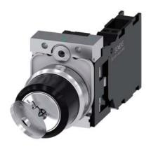
RONIS key-operated switch, 22 mm, round, metal, shiny, lock number SB30, with 2 keys, 2 switch positions O-I, latching, actuating angle 90°, 10:30h/13:30h, key removal O+I, with holder, 1 NO+1 NC, spring-type terminal, possible special locks: SB31, 421, 455
