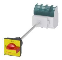
SENTRON, switch disconnector 3LD, EMERGENCY OFF switch, 4-pole, lu: 63 A, Operating power / at AC-23 A at 400 V: 22 kW, floor mounting with door coupling, defeatable knob-operated mechanism, red/yellow, 4-hole mounting of the handle
