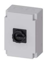
SENTRON, Switch disconnector 3LD, main switch, 3-pole, lu: 100 A, Operating power / at AC-23 A at 400 V: 37 kW, molded-plastic encapsulation for inch cable gland, rotary operating mechanism, black
