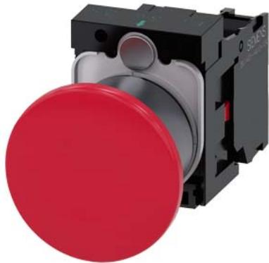
Mushroom pushbutton, 22 mm, round, plastic with metal front ring, red, 40mm, latching, pull-to-unlatch mechanism, with holder, 1 NC, screw terminal, with laser labeling, symbol number according to, ISO 7000 or IEC 60417
