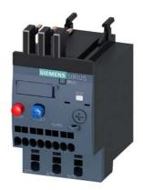
Overload relay 0.28...0.40 A Thermal For motor protection Size S00, Class 10 Contactor mounting Main circuit: Spring-type terminal Auxiliary circuit: spring-type terminal Manual-Automatic-Reset
