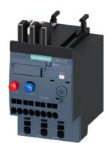
Overload relay 0.70...1.0 A Thermal For motor protection Size S00, Class 10 Contactor mounting Main circuit: Spring-type terminal Auxiliary circuit: spring-type terminal Manual-Automatic-Reset
