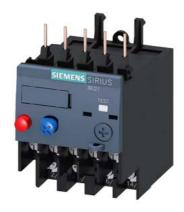
Overload relay 5.5...8.0 A Thermal For motor protection Size S00, Class 10 Contactor mounting Main circuit: Ring cable lug Auxiliary circuit: ring cable lug Manual-Automatic-Reset
