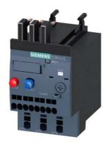
Overload relay 0.14...0.20 A Thermal For motor protection Size S00, Class 10 Contactor mounting Main circuit: Spring-type terminal Auxiliary circuit: spring-type terminal Manual-Automatic-Reset
