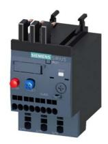
Overload relay 4.5...6.3 A Thermal For motor protection Size S00, Class 10 Contactor mounting Main circuit: Spring-type terminal Auxiliary circuit: spring-type terminal Manual-Automatic-Reset
