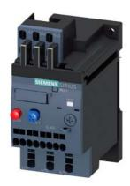
Overload relay 0.45...0.63 A Thermal For motor protection Size S00, Class 10 Stand-alone installation Main circuit: Spring-type terminal Auxiliary circuit: spring-type terminal Manual-Automatic-Reset
