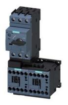
Load feeder fuseless, Reversing duty 400 V AC, Size S00 4.50...6.30 A 230 V AC screw terminal for installation on standard mounting rail Type of coordination 1, Iq = 150 kA 1 NC (contactor)
