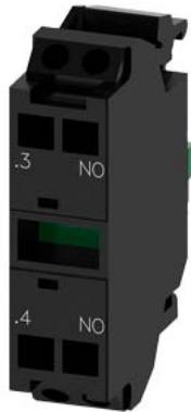
Contact module with 1 contact element, 1 NO, spring-type terminal, for front plate mounting, Z=150-unit packaging
