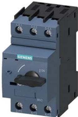
Circuit breaker size S00 for starter combination Rated current 0.4 A N-release 5.2 A screw terminal Standard switching capacity
