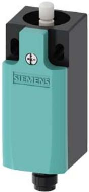
position switch plastic enclosure according to EN 50047, 31 mm 1 NO/1 NC quick action contacts integrated (not replaceable) with M12 connector, 4-pole pin assignment: Pin1=21, Pin2=22 Pin3=13, Pin4=14 for max. 250 V and 4 A, with rounded plunger
