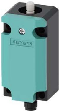
Position switch Plastic enclosure 40 mm according to EN 50041 1 NO/1 NC quick action contacts with M12 connector, 4-pole Pin assignment: Pin1=21, Pin2=22 PIN3=13, PIN4=14 max. 250 V and 4 A Teflon plunger
