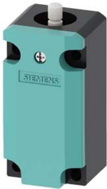
Basic switch for position switch 3SE513 Enclosure plastic according to EN 50041, 1 x (M20 x 1.5) 1 NO/1 NC slow-action contacts without actuator head
