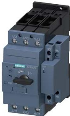
Circuit breaker size S2 for motor protection, CLASS 10 with overload relay function A-release 28...36 A N-release 520 A Standard switching capacity
