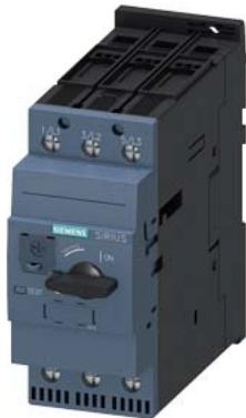
Circuit breaker size S2 for transformer protection A-release 54...65 A N-release 1040 A screw terminal Standard switching capacity
