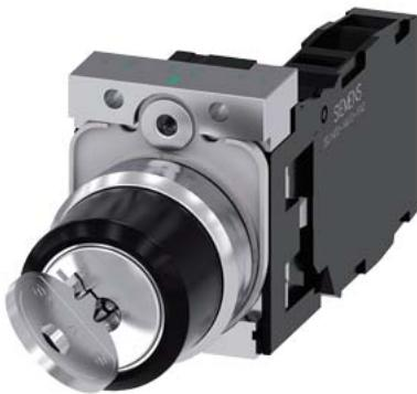
RONIS key-operated switch, 22 mm, round, metal, shiny, lock number SB30, with 2 keys, 2 switch positions O-I, latching, actuating angle 90°, 10:30h/13:30h, key removal O+I, with holder, 1 NO+1 NC, screw terminal, possible special locks: SB31, 421, 455 lower case
