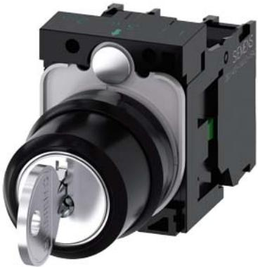
RONIS key-operated switch, 22 mm, round, plastic, lock number SB30, with 2 keys, 3 switch positions I-O-II, latching, 10:30h/12h/13:30h, Key removal I+O+II, with holder, 1 NO, 1 NO, screw terminal, possible special locks: SB31, 421, 455, with laser labeling, inscription or symbol Customer-specific selection with SIRIUS ACT configurator (CIN)
