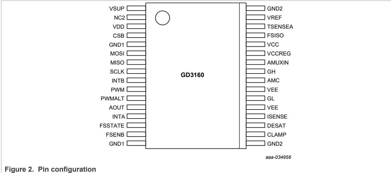
Figure 2. Pin configuration
