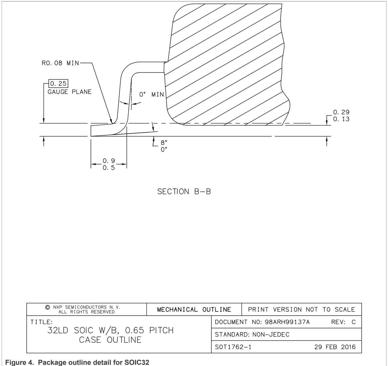
Figure 4. Package outline detail for SOIC32
