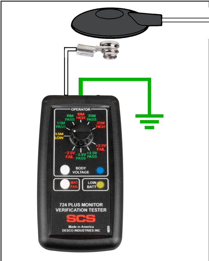
Figure 5. Connecting the 724 Plus Monitor Verification Tester to the 724 Plus Workstation Monitor's mat monitor cord
