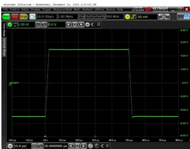
Figure 23 Large-Signal Pulse Response Voltage: 2V/div for Output, Time: 10us/div G=1, VREF = GND; VIN=10VPP, Load R=10K C=100pF
