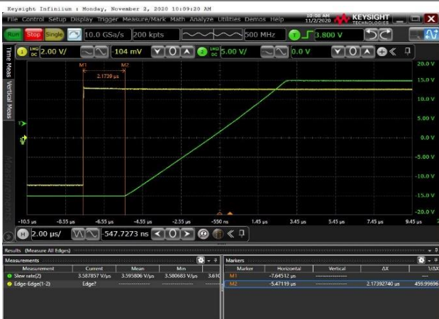
Figure 21 Positive Overload Recovery Voltage: 5V/div for Output, Time: 2us/div G=10, VREF = GND; VIN=10VPP, Load R=10K C=100pF
