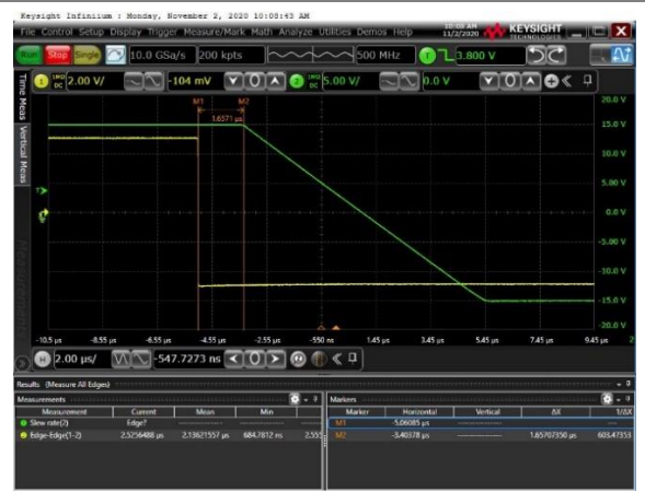
Figure 22 Negative Overload Recovery Voltage: 5V/div for Output, Time: 2us/div G=10, VREF = GND; VIN=10VPP, Load R=10K C=100pF
