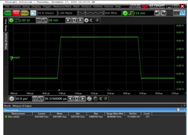
Figure 20 Slew Rate Voltage: 2V/div for Output, Time: 10us/div G=1, VREF = GND; VIN=10VPP, Load R=10K
