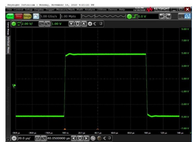
Figure 24 Large-Signal Pulse Response Voltage: 2V/div for Output, Time: 20us/div G=10, VREF = GND; VIN=1VPP, Load R=10K C=100pF
