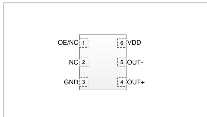
Figure 2. Pin Assignments (Top view)
