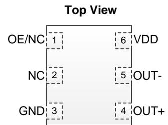
**Figure 3. Pin Assignments**
