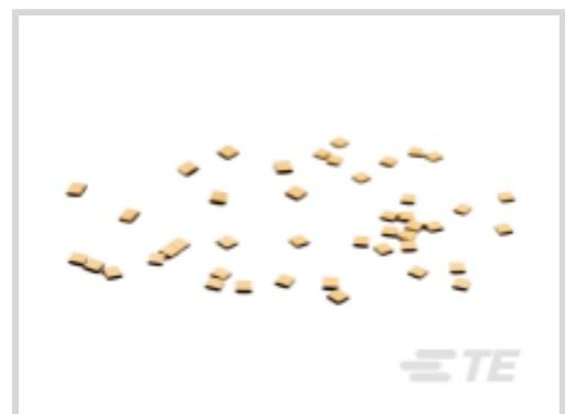
Discrete NTC Sensor Type: **Leadless NTC Gold Chips**Wire Connection: **Solder/Wire Bond**Resistance (at 25°C): **10 kΩ**Tolerance Resistance: **± 2 %, ± 2 %**β-Value(25/85): **3976 K**[All Gold Chip NTC Thermistors \(10\)](#)
