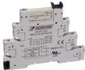
Plug-Relay-Compact (PRC) Complete, Consisting of base PRC... with screw connection and pluggable miniature relay PRC... with power contact, Mounting type: Mounting rail TS 35, 1 CO contact, Input voltage: 12 VDC
