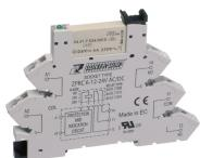
Plug-Relay-Compact (PRC) socket base PRC with tension-spring connection, Mounting type: Mounting rail TS 35, 1 CO contact, Input voltage: 6, 12 or 24 VAC/DC
