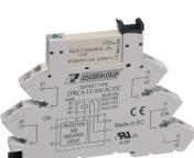
Plug-Relay-Compact (PRC) Complete, Consisting of base PRC... with screw connection and pluggable miniature relay PRC... with power contact, Mounting type: Mounting rail TS 35, 1 CO contact, Input voltage: 60 VAC/DC
