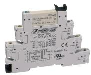
Plug-Relay-Compact (PRC) socket base PRC with screw connection, Mounting type: Mounting rail TS 35, 1 CO contact, Input voltage: 6, 12 or 24 VDC
