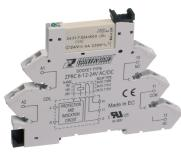
Plug-Relay-Compact (PRC) Complete, Consisting of base PRC... with tension-spring connection and pluggable miniature relay PRC... with power contact, Mounting type: Mounting rail TS 35, 1 CO contact, Input voltage: 125 VAC/DC
