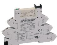
Plug-Relay-Compact (PRC) socket base PRC with tension-spring connection, Mounting type: Mounting rail TS 35, 1 CO contact, Input voltage: 110 to 125 VAC/DC
