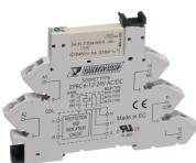
Plug-Relay-Compact (PRC) Complete, Consisting of base PRC... with screw connection and pluggable miniature relay PRC... with power contact, Mounting type: Mounting rail TS 35, 1 CO contact, Input voltage: 125 VAC/DC
