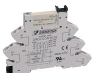
Plug-Relay-Compact (PRC) socket base PRC with tension-spring connection and residual current suppression for long cables, Mounting type: Mounting rail TS 35, 1 CO contact, Input voltage: 220 to 240 VAC
