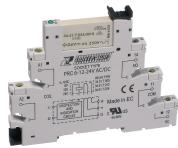
Plug-Relay-Compact (PRC) Complete, Consisting of base PRC... with screw connection and pluggable miniature relay PRC... with power contact, Mounting type: Mounting rail TS 35, 1 CO contact, Input voltage: 24 VDC
