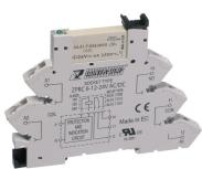
Plug-Relay-Compact (PRC) socket base PRC with tension-spring connection and residual current suppression for long cables, Mounting type: Mounting rail TS 35, 1 CO contact, Input voltage: 110 to 125 VAC/DC
