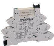
Plug-Relay-Compact (PRC) Complete, Consisting of base PRC... with screw connection and pluggable miniature relay PRC... with power contact, Mounting type: Mounting rail TS 35, 1 CO contact, Input voltage: 24 VDC
