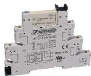
Plug-Relay-Compact (PRC) Complete, Consisting of base PRC... with screw connection and pluggable miniature relay PRC... with power contact, Mounting type: Mounting rail TS 35, 1 CO contact, Input voltage: 240 VAC/DC
