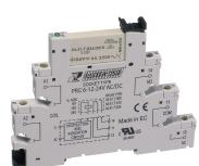
Plug-Relay-Compact (PRC) socket base PRC with screw connection and residual current suppression for long cables, Mounting type: Mounting rail TS 35, 1 CO contact, Input voltage: 220 to 240 VAC
