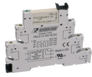
Plug-Relay-Compact (PRC) Complete, Consisting of base PRC... with screw connection and pluggable miniature relay PRC... with power contact, Mounting type: Mounting rail TS 35, 1 CO contact, Input voltage: 6 VDC
