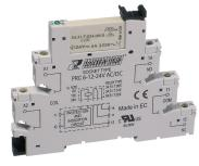
Plug-Relay-Compact (PRC) socket base PRC with screw connection, Mounting type: Mounting rail TS 35, 1 CO contact, Input voltage: 220 to 240 VAC/DC
