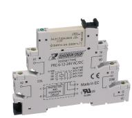
Plug-Relay-Compact (PRC) socket base PRC with screw connection and residual current suppression for long cables, Mounting type: Mounting rail TS 35, 1 CO contact, Input voltage: 110 to 125 VAC/DC
