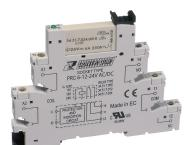
Plug-Relay-Compact (PRC) socket base PRC with screw connection, Mounting type: Mounting rail TS 35, 1 CO contact, Input voltage: 110 to 125 VAC/DC
