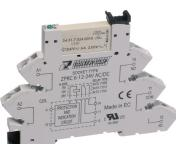
Plug-Relay-Compact (PRC) Complete, Consisting of base PRC... with tension-spring connection and pluggable miniature relay PRC... with power contact, Mounting type: Mounting rail TS 35, 1 CO contact, Input voltage: 12 VAC/DC
