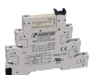
Plug-Relay-Compact (PRC) Complete, Consisting of base PRC... with screw connection and pluggable miniature relay PRC... with power contact, Mounting type: Mounting rail TS 35, 1 CO contact, Input voltage: 48 VAC/DC
