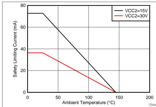
**Figure 1. Thermal Derating Curve for Limiting Current per VDE for D Package**
