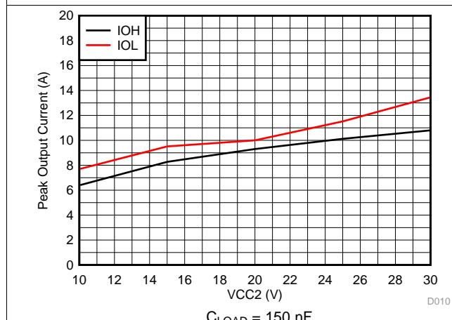
**Figure 7. UCC5350SBD Output-High Drive Current vs Output Voltage**
