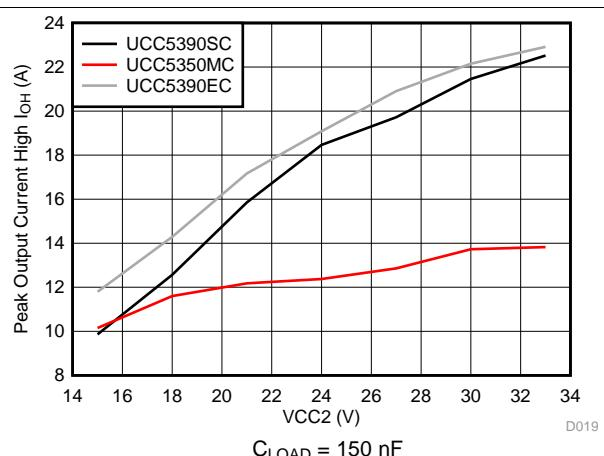
**Figure 6. Output-High Drive Current vs Output Voltage**
