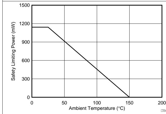
**Figure 3. Thermal Derating Curve for Limiting Power per VDE for D Package**
