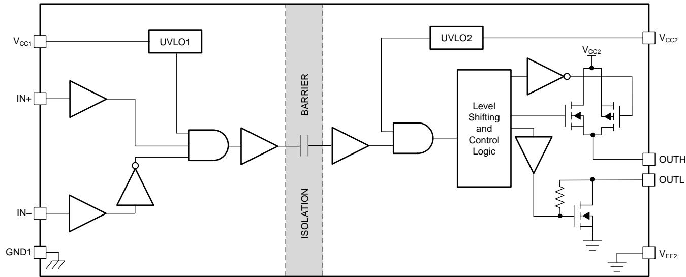
**Figure 49. Functional Block Diagram — Split Output (UCC53x0S)**
