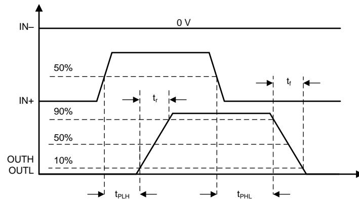
Figure 42. OUTH and OUTL Propagation Delay, Noninverting Configuration
