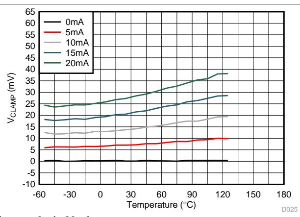
**Figure 24.  $V_{Clamp}$  vs Temperature**
