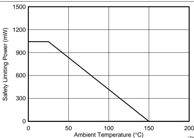
**Figure 4. Thermal Derating Curve for Limiting Power per VDE for DWV Package**
