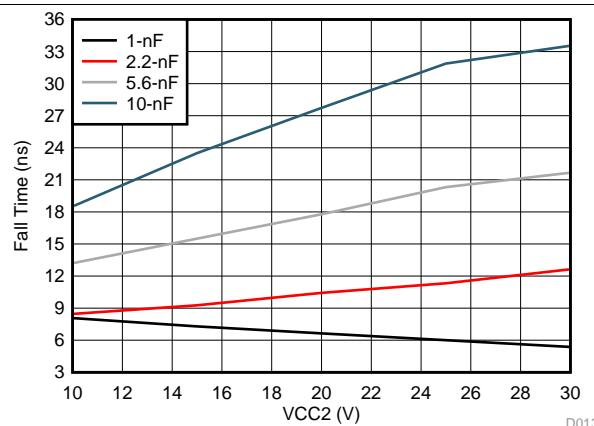
Figure 41. UCC5350SBD Fall Time vs  $C_L$  and  $V_{CC2}$
