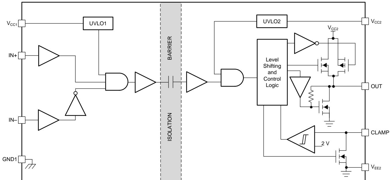
**Figure 50. Functional Block Diagram — Miller Clamp (UCC53x0M)**
