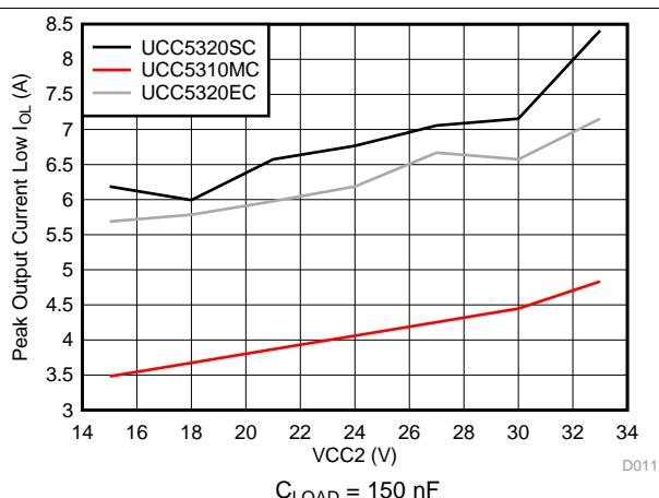
**Figure 8. Output-Low Drive Current vs Output Voltage**
