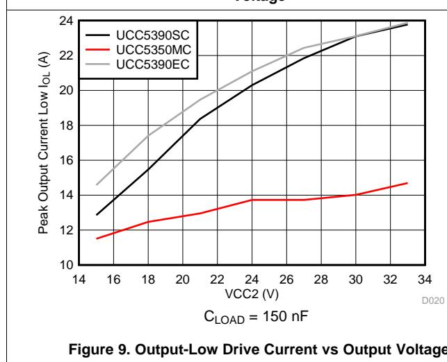
**Figure 9. Output-Low Drive Current vs Output Voltage**
