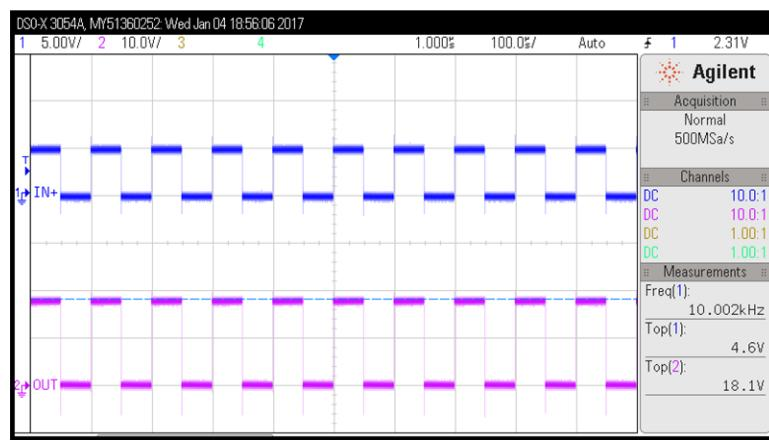
$$V_{CC2} = 20 \text{ V} \quad V_{EE2} = \text{GND} \quad f_{SW} = 10 \text{ kHz}$$
