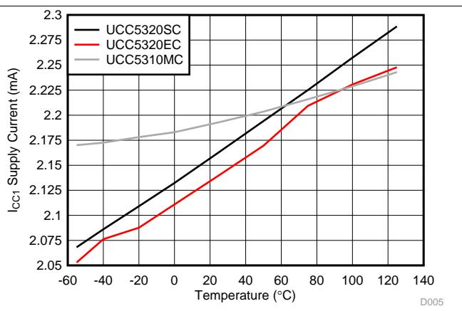
Figure 12.  $I_{CC1}$  Supply Current vs Temperature
