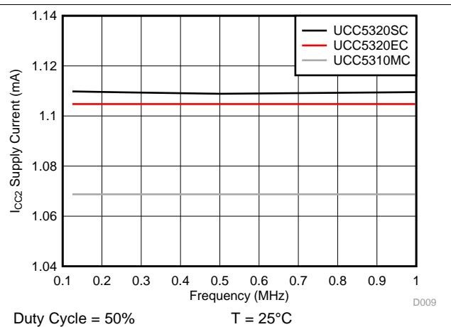
Figure 20.  $I_{CC2}$  Supply Current vs Input Frequency
