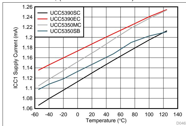
Figure 11.  $I_{CC1}$  Supply Current vs Temperature
