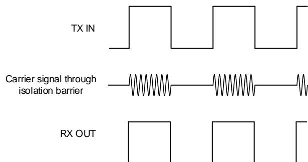
**Figure 48. On-Off Keying (OOK) Based Modulation Scheme**
