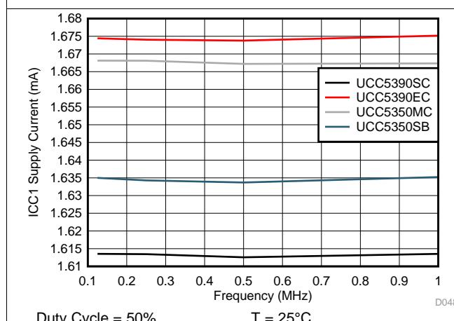
Figure 15.  $I_{CC1}$  Supply Current vs Input Frequency
