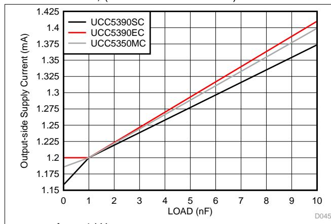
**Figure 23.  $I_{CC2}$  Supply Current vs Load Capacitance**
