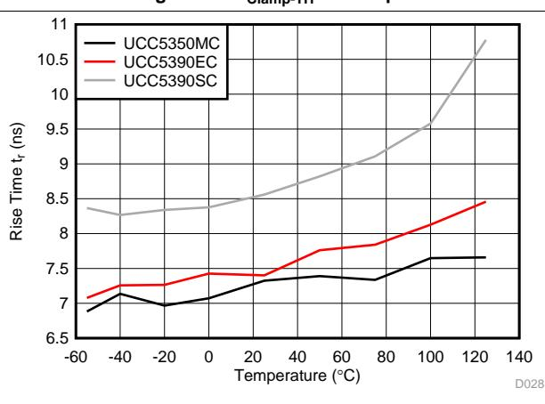
**Figure 28. Rise Time vs Temperature**
