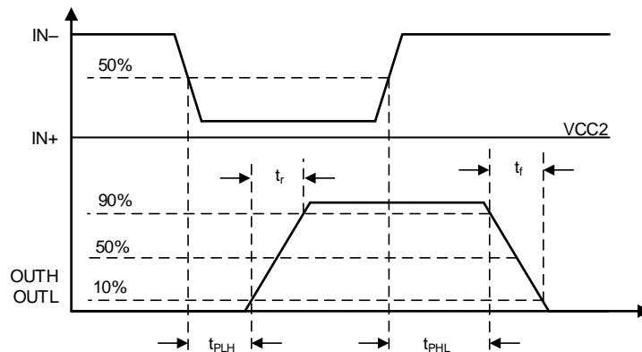
Figure 43. OUTH and OUTL Propagation Delay, Inverting Configuration
