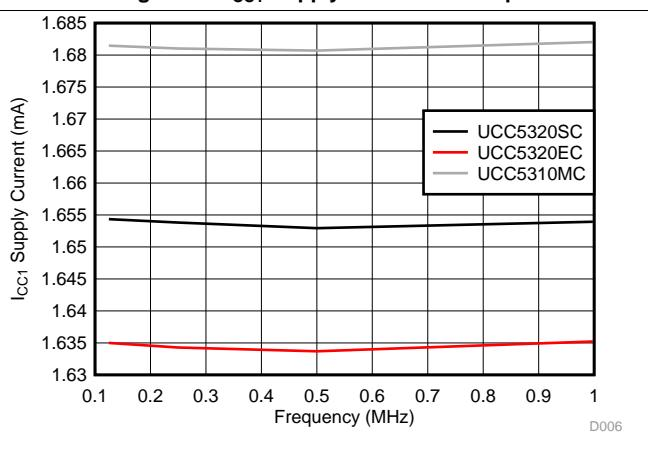
Figure 14.  $I_{CC1}$  Supply Current vs Input Frequency
