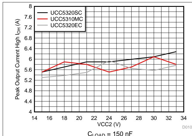
**Figure 5. Output-High Drive Current vs Output Voltage**
