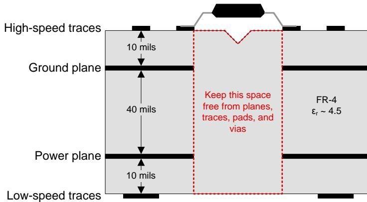
**Figure 67. Recommended Layer Stack**
