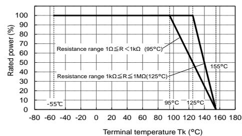
Fig.4< Terminal temperature >
