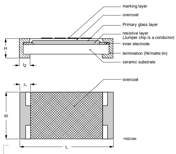
Fig. 5 Chip resistor outlines
