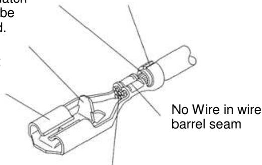
No Wire in wire barrel seam
