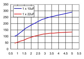
Figure 26. Input ripple voltage for various outputs with a 10  $\mu F$  or a 22  $\mu F$  ceramic capacitor at the input (full-load).
