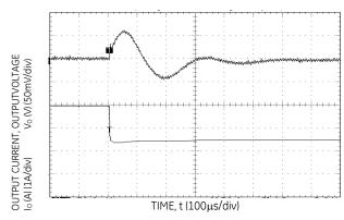
Figure 13. Transient Response to Dynamic Load Change from 100% of 50% full load (Vo = 3.3Vdc, Cext =  $2x150~\mu F$  Polymer Capacitors).
