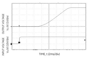
Figure 16. Typical Start-Up with application of Vin (VIN = 12.0Vdc, Vo = 3.3Vdc, Io = 3A).
