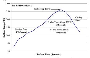
Figure 36. Recommended linear reflow profile using Sn/Ag/Cu solder.
