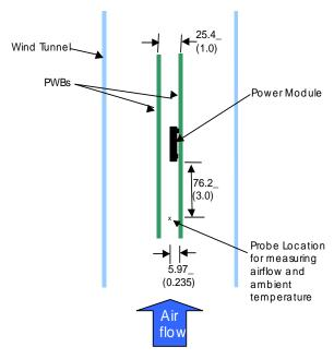
Figure 32. Thermal Test Set-up.
