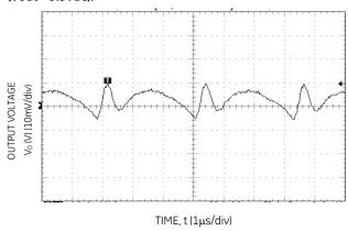
Figure 8. Typical Output Ripple and Noise (Vin = 12.0V dc, Vo = 0.75Vdc, Io=3A).
