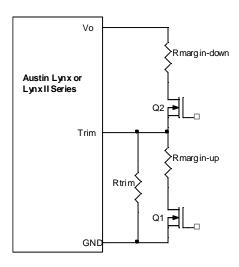
Figure 30. Circuit Configuration for margining Output voltage.
