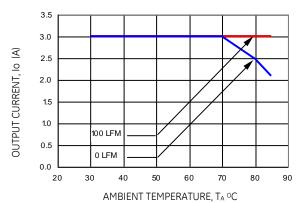
Figure 21. Derating Output Current versus Local Ambient Temperature and Airflow ( $V_{\rm IN}=12.0 Vdc$ , Vo=3.3 Vdc).
