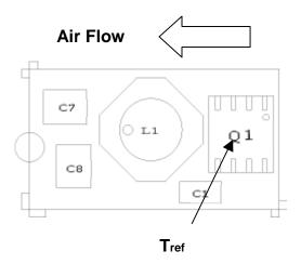
Figure 31. Tref Temperature measurement location.
