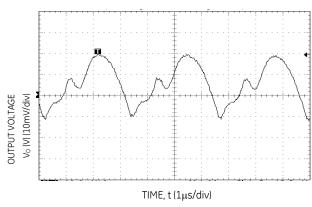
Figure 9. Typical Output Ripple and Noise (VIN = 12.0V dc, Vo = 3.3Vdc, Io=3A).
