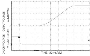
Figure 15. Typical Start-Up Using Remote On/Off with Low-ESR external capacitors (7x150uF Polymer)
