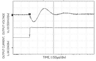
Figure 12. Transient Response to Dynamic Load Change from 50% to 100% of full load (Vo = 3.3 Vdc, Cext = 2x150  $\mu F$  Polymer Capacitors).
