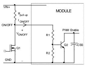
Figure 28. Circuit configuration for using negative logic On/OFF.
