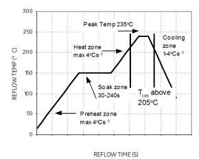
Figure 34. Reflow Profile for Tin/Lead (Sn/Pb) process.
