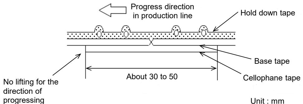
b) When hold down tape is spliced
