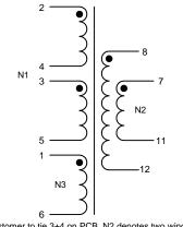
Customer to tie 3+4 on PCB. N2 denotes two windings connected in parallel. Terminals 7+8, 11+12 must be tied as solder bridging is allowed.
