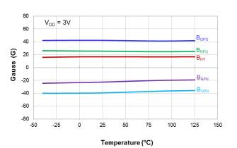
Switch Points Bops and BRPS vs Temperature
