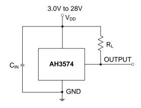
Note: 4.  $C_{IN}$  is for power stabilization and to strengthen the noise immunity, the recommended capacitance is 10nF ~ 100nF. R<sub>L</sub> is the pull-up resistor.
