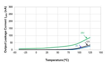
Output Leakage Current vs Temperature
