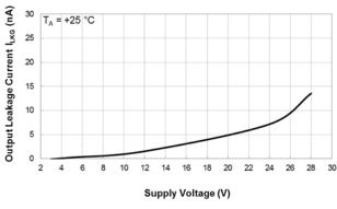
Output Leakage Current vs Supply Voltage
