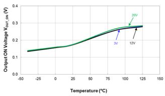
Output ON Voltage vs Temperature
