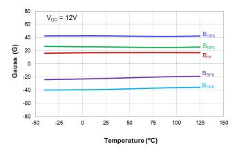
Switch Points B<sub>OPS</sub> and B<sub>RPS</sub> vs Temperature
