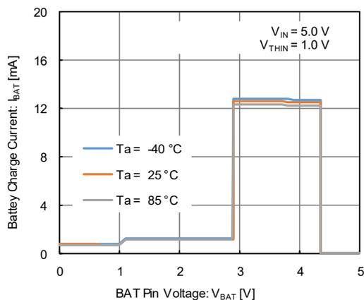
(5) Battery Charge Current vs. BAT Pin Voltage
