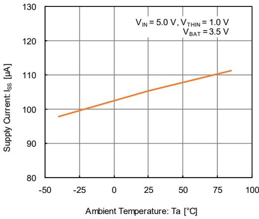
(8) Standby Current vs. Ambient Temperature
