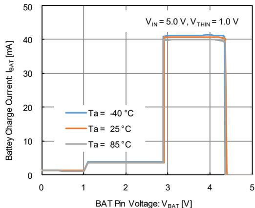
(6) Charge Completion Current vs. Ambient Temperature
