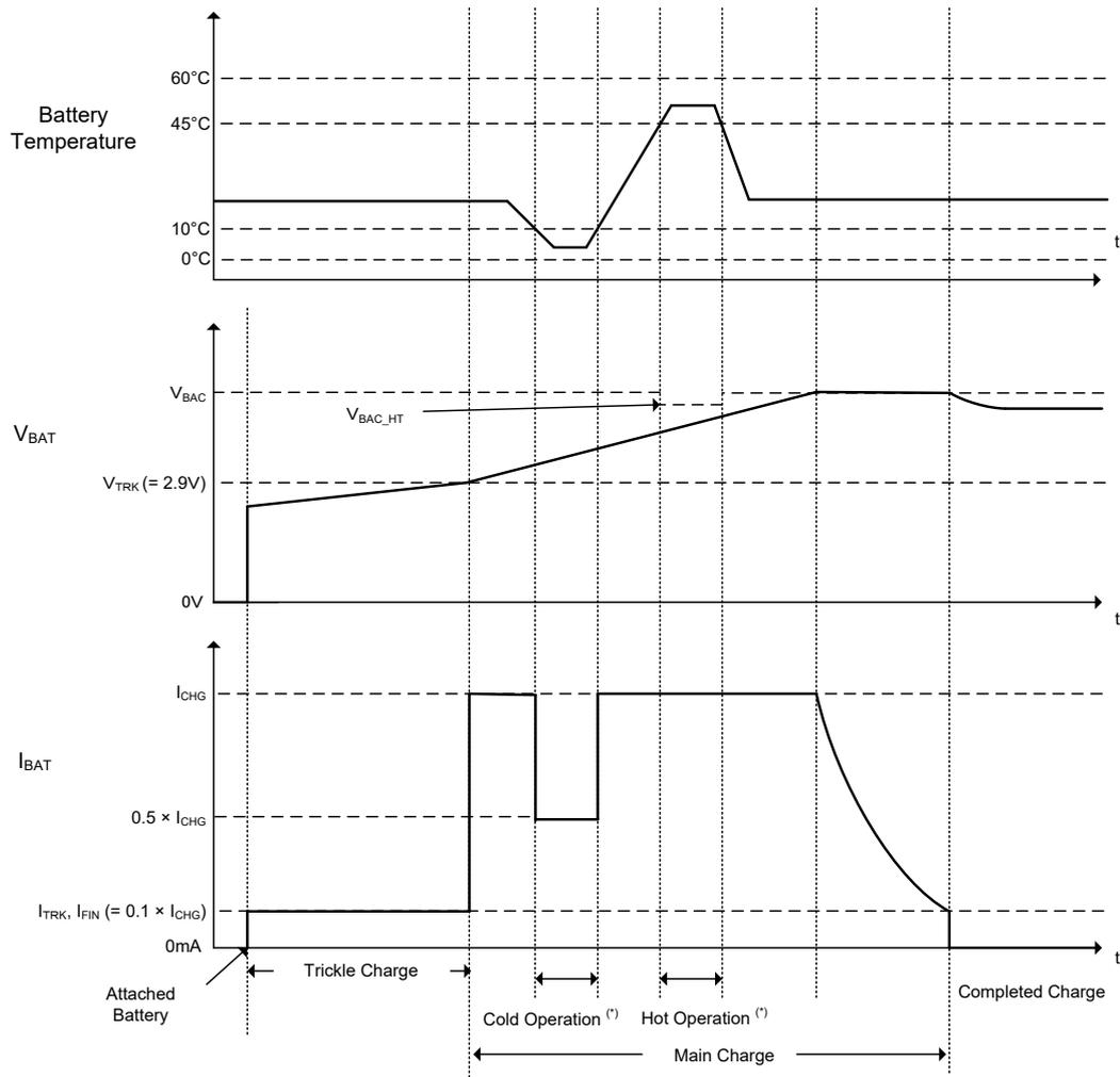
(\* ) With regard to the details of Cold operation and Hot Operation, please see "Li-ion battery temperature monitoring function" in the Operational Explanation.
