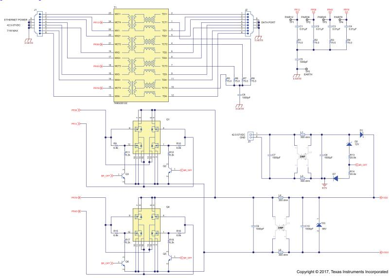
Figure 1. TPS2372-4EVM-006 Front End Interface Schematic
