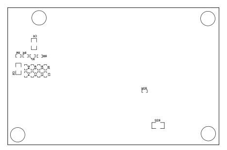
**Figure 12. Bottom Component Placement**
