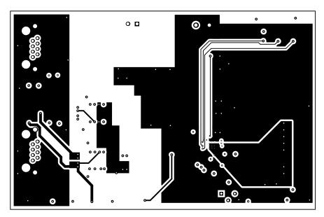
Figure 10. Layer 3 Routing
