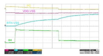
Figure 5. Current-Limit Protection Performance
