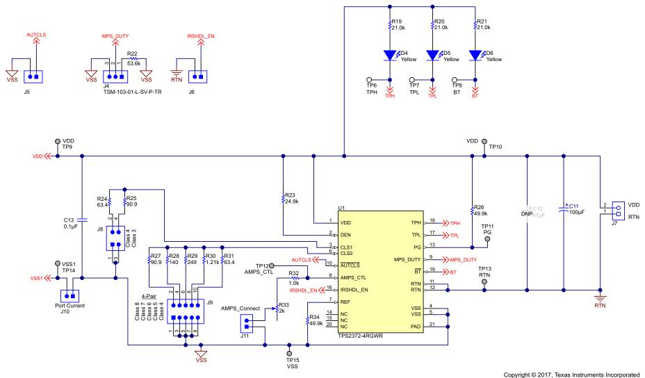
Figure 2. TPS2372-4EVM-006 PD Controller Schematic
