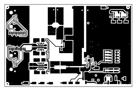
Figure 8. Top Side Routing
