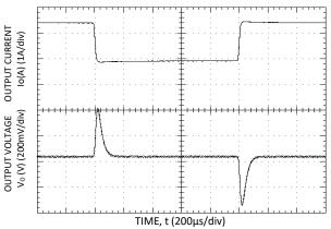
Figure 4. Transient Response to 0.1A/ $\mu$ S Dynamic Load Change from 50% to 75% to 50% of full load, Vin=48V,  $C_0>100\mu F$ .
