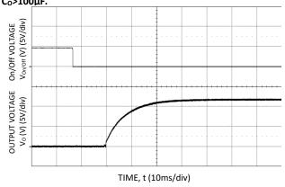
Figure 5. Typical Start-up Using Remote On/Off, negative logic version shown ( $V_{IN} = 24V$  or 48V,  $I_0 = I_{0,max}$ ).
