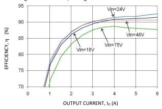
Figure 1. Converter Efficiency versus Output Current.
