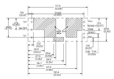
TH Recommended Pad Layout (Component Side View)
