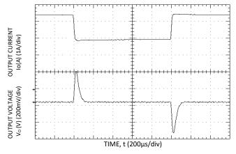
Figure 3. Transient Response to  $0.1A/\mu S$  Dynamic Load Change from 50% to 75% to 50% of full load, Vin=24V,  $C_0>100\mu F$ .
