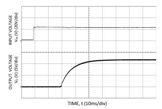
Figure 6. Typical Start-up Using Input Voltage ( $V_{IN}$  = 24V,  $I_0$  =  $I_{O,max}$ ).
