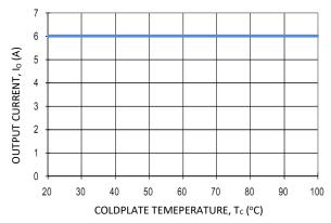
Figure 20. Derated Output Current versus Cold Wall Temperature with Local Ambient Temperature Around Module at 85C;  $V_{\rm IN}$  =24V or 48V.
