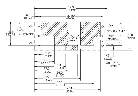
TH Recommended Pad Layout (Component Side View)
