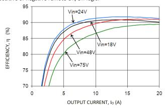
Figure 1. Converter Efficiency versus Output Current.
