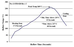
Figure 27. Recommended linear reflow profile using Sn/Ag/Cu solder.
