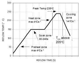
Figure 25. Reflow Profile for Tin/Lead (Sn/Pb) process.
