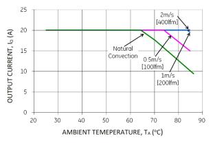
Figure 21. Output Current Derating for the Module with-18 Heatplate; Airflow in the Transverse Direction from  $V_{out}(-)$  to  $V_{out}(+)$ ;  $V_{IN} = 24V$ .
