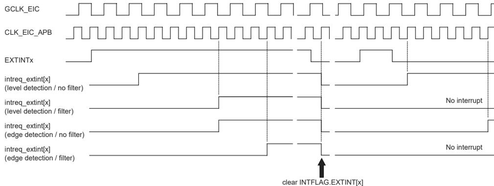
Detection latency depends on the detection mode.
