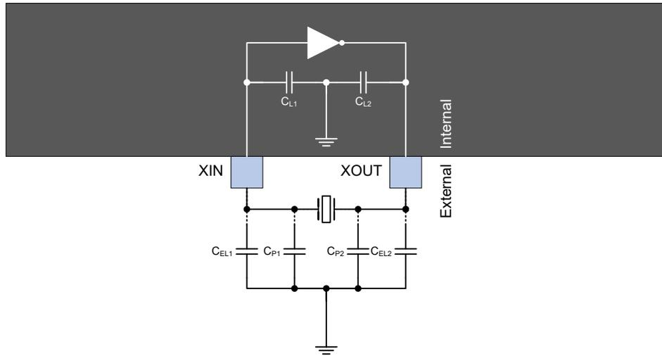
Using this model, the total capacitive load for the crystal can be calculated as shown in the equation below:
