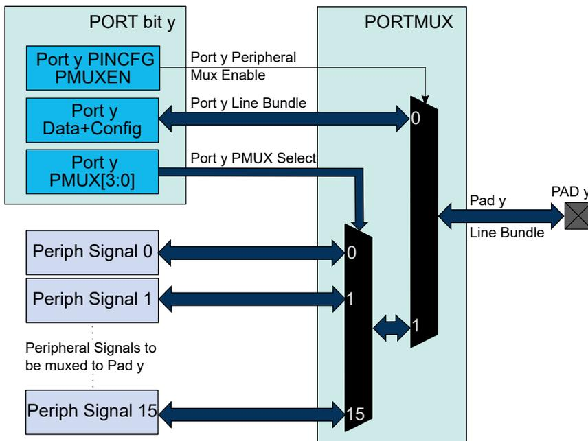
The I/O pins of the device are controlled by the PORT peripheral registers. Each port pin has a corresponding bit in the Data Direction (DIR) and Data Output Value (OUT) registers to enable that pin as an output and to define the Output state.
