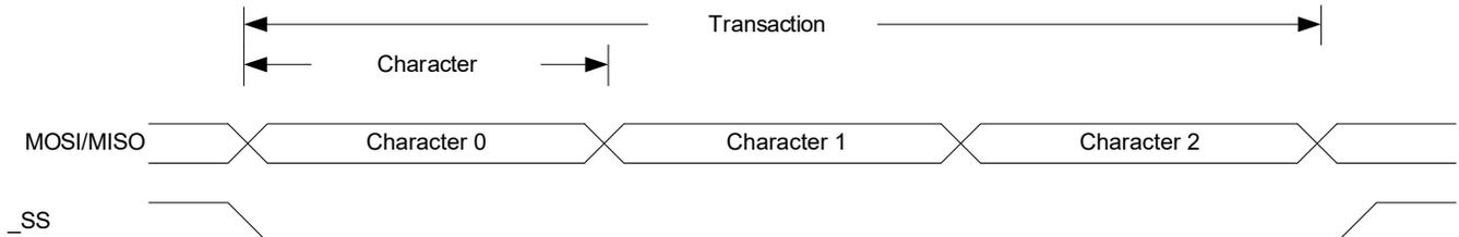
The SPI host must pull the SPI select line ( $\overline{SS}$ ) of the desired client low to initiate a transaction if multiple clients are connected to the bus. The SPI select line can be wired low if there is only one SPI client on the bus. The host and client prepare data to send via their respective Shift registers, and the host generates the serial clock on the SCK line.
