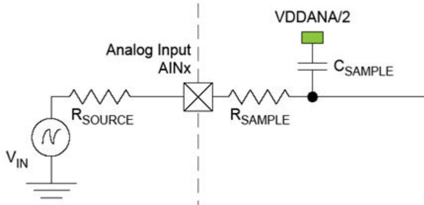
The minimum sampling time  $t_{\text{samplehold}}$  for a given  $R_{\text{source}}$  can be calculated using this formula:
