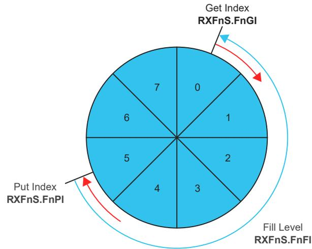
When reading from an Rx FIFO, Rx FIFO Get Index  $RXFnS.FnGI \cdot \text{FIFO Element Size}$  has to be added to the corresponding Rx FIFO start address  $RXFnC.FnSA$ .
