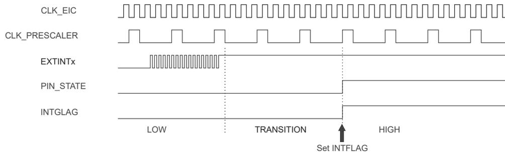
In the Synchronous Edge Detection mode, the EIC clock is required. The Synchronous Edge Detection mode can be used in Idle and Standby Sleep modes.
