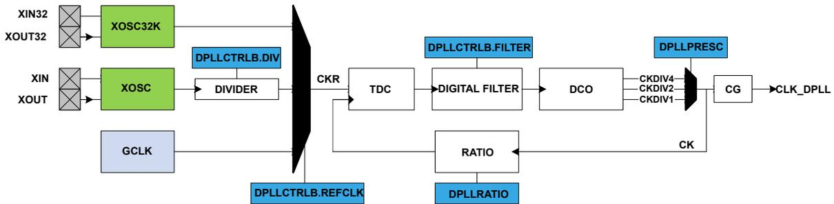
When the controller is disabled, the output clock is low. If the Loop Divider Ratio Fractional part bit field in the DPLL Ratio register (**DPLLCTRLB.LDRFRAC**) is zero, the DPLL works in integer mode. Otherwise, the fractional mode is activated. Note that the fractional part has a negative impact on the jitter of the DPLL.
