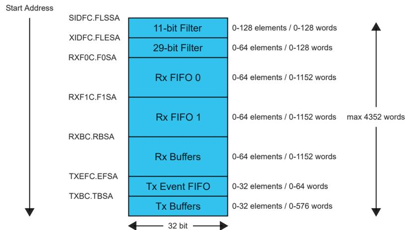
When the CAN addresses the Message RAM it addresses 32-bit words, not single bytes. The configurable start addresses are 32-bit word addresses (i.e. only bits 15 to 2 are evaluated and the two LSBs are ignored).
