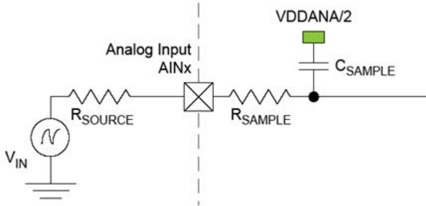
The minimum sampling time  $t_{\text{samplehold}}$  for a given  $R_{\text{source}}$  can be found using this formula:
