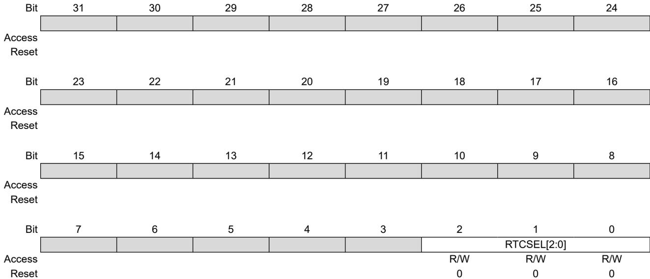
**Bits 2:0 – RTCSEL[2:0]** RTC Clock Source Selection
