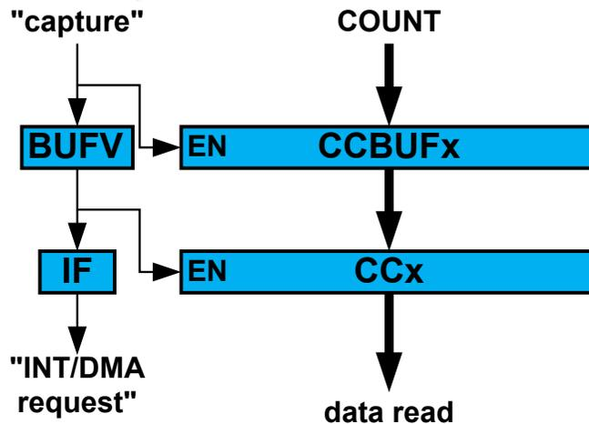
The TCC can detect capture overflow of the input capture channels: When a new capture event is detected while the Capture Buffer Valid flag (STATUS.CCBUFV) is still set, the new timestamp will not be stored and INTFLAG.ERR will be set.
