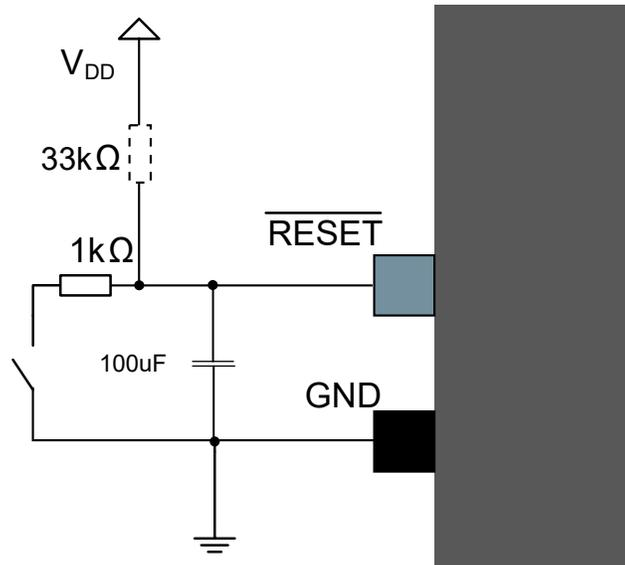
**Figure 53-6. External Reset Circuit Schematic (EFT Immunity Enhancement)**
