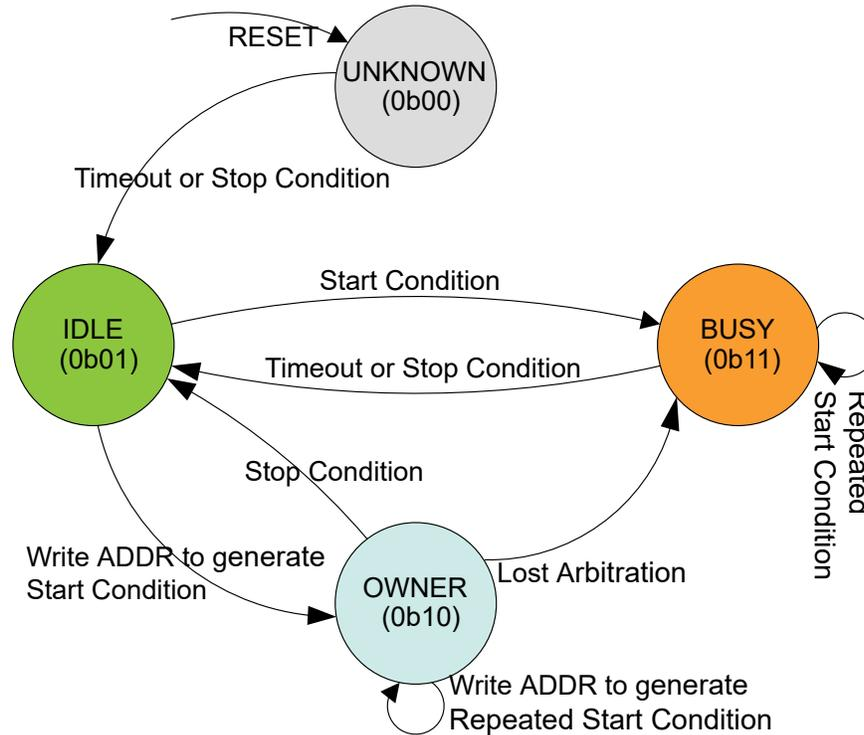
The Bus state machine is active when the I<sup>2</sup>C host is enabled.
