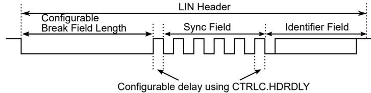
After header transmission is complete, the Client responds with 1-8 data bytes plus checksum.
