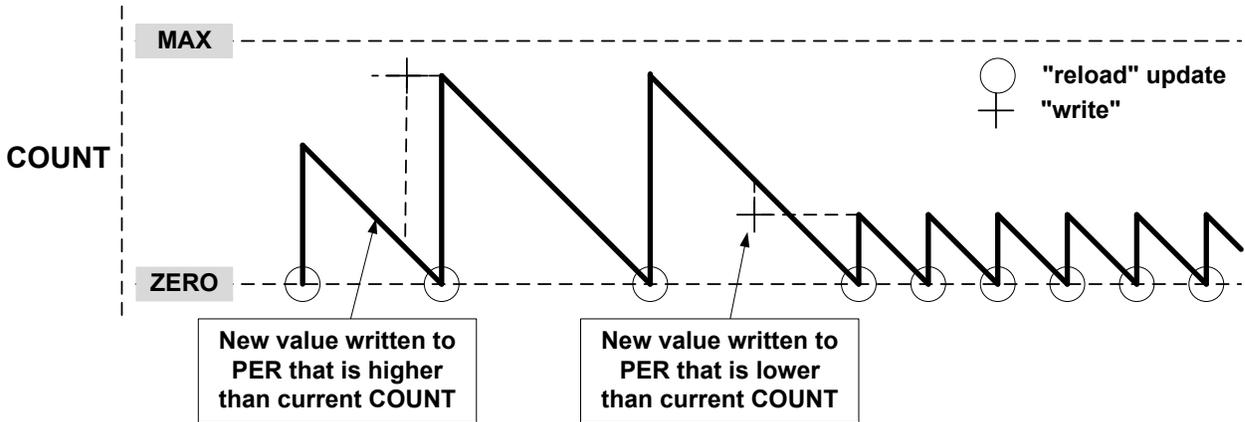
A counter wraparound can occur in any operation mode when up-counting without buffering, see [Figure 36-10](#). COUNT and TOP are continuously compared, so when a new value that is lower than the current COUNT is written to TOP, COUNT will wrap before a compare match.
