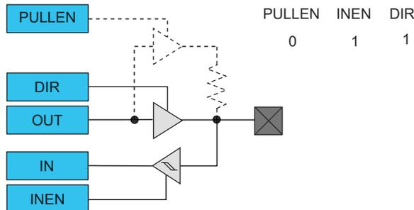
**Figure 28-8. I/O Configuration - Output with Pull**
