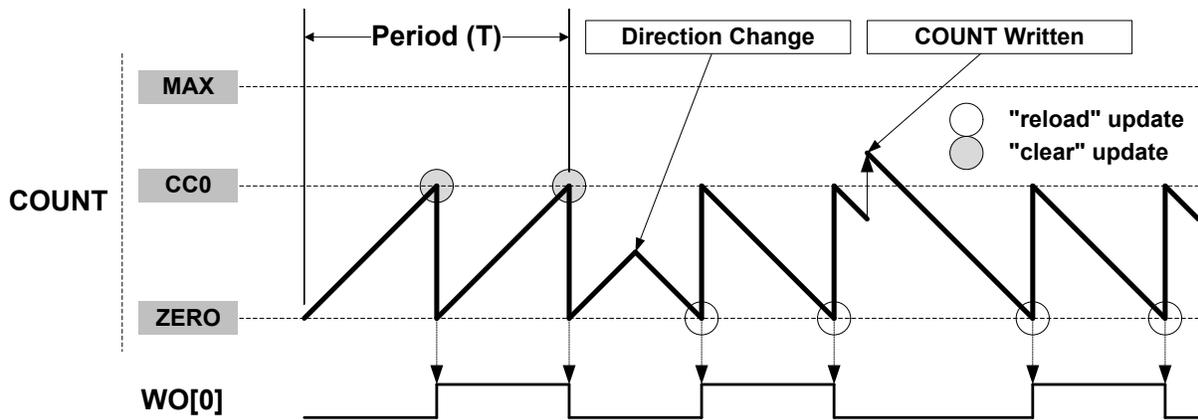
**Normal Pulse-Width Modulation Operation (NPWM)**
