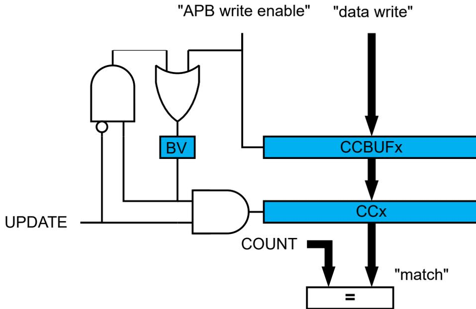
Both the registers (PATT/WAVE/PER/CCx) and corresponding buffer registers (PATTBUF/WAVEBUFV/PERBUF/CCBUFx) are available in the I/O register map, and the double buffering feature is not mandatory. The double buffering is disabled by writing a '1' to CTRLSET.LUPD.
