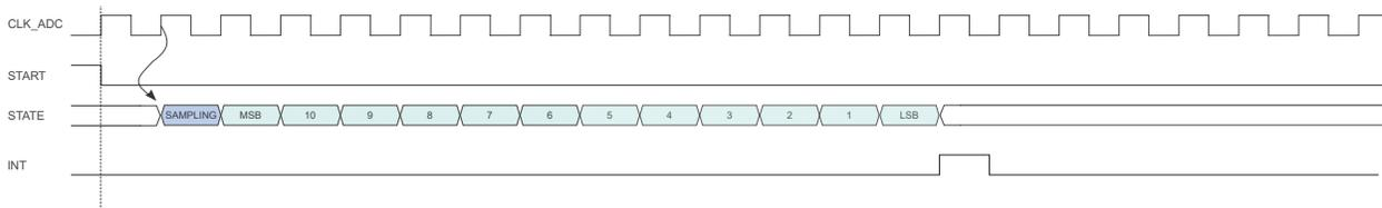
The sampling time can be increased by using the Sampling Time Length bit group in the Sampling Time Control register (SAMPCTRL.SAMPLEN). As example, the next figure is showing the timing conversion with sampling time increased to six CLK\_ADC cycles.
