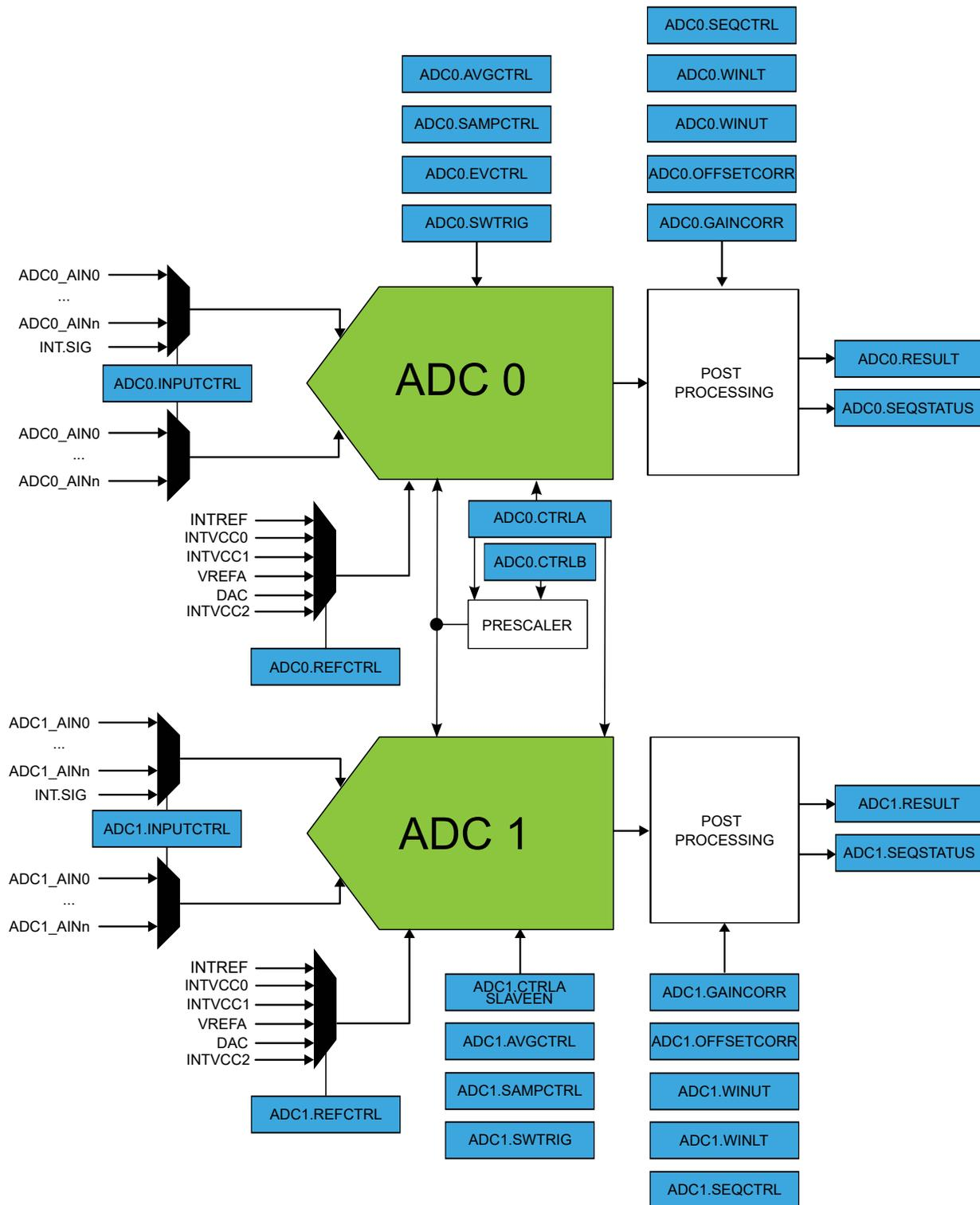
In this mode of operation, the Client ADC is enabled by accessing the CTRLA register of Host ADC. In the same way, the Host ADC event inputs will be automatically routed to the Client ADC, meaning that the input events configuration must be done in the Host ADC (ADC0.EVCTRL).
