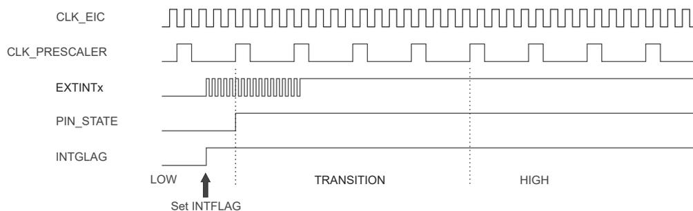
In this mode, the EIC clock is requested. The asynchronous Edge Detection mode can be used in Idle and Standby Sleep modes.
