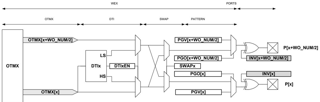
The output matrix (OTMX) unit distributes compare channels, according to the selectable configurations in Table 36-4.
