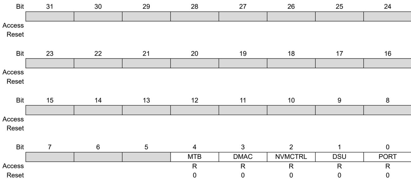
**Bit 4 – MTB** Peripheral MTB Write Protection Status
