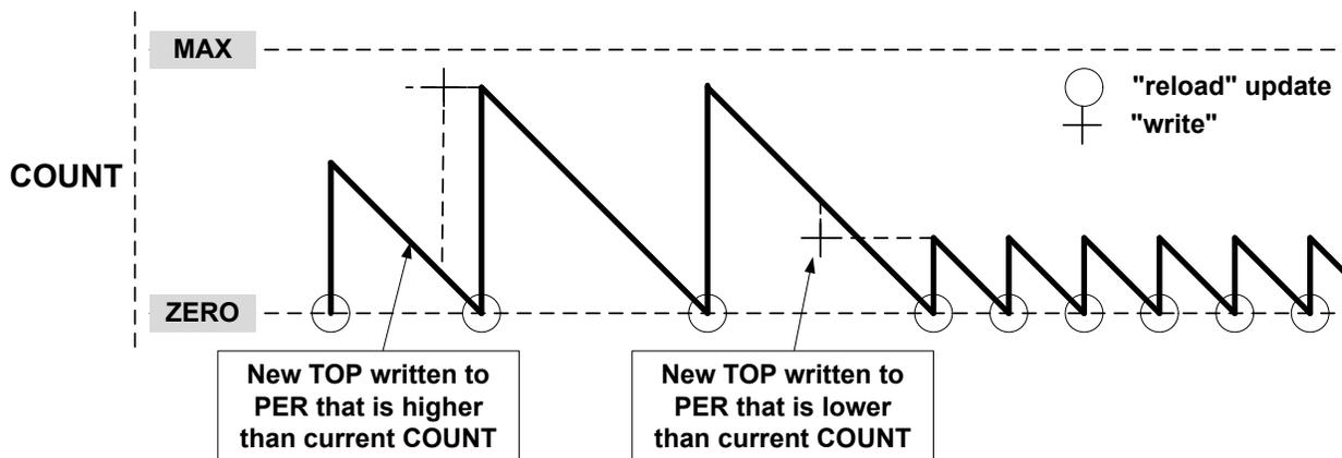
When double buffering is used, the buffer can be written at any time and the counter will still maintain correct operation. The period register is always updated on the update condition, as shown in [Figure 35-10](#). This prevents wraparound and the generation of odd waveforms.
