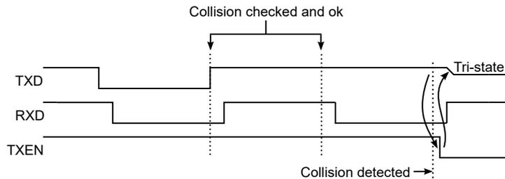
When a collision is detected, the USART follows this sequence:
