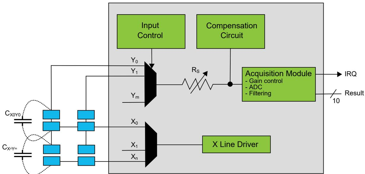
**Note:** For SAM C20/C21 the  $R_s = 0, 20, 50, 100 \text{ K}\Omega$ .
