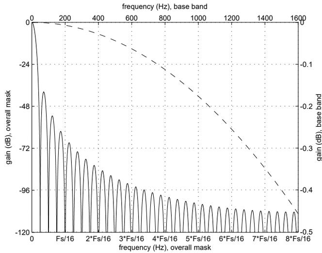
The zeros of this filter are located at multiples of CLK\_SDADC\_FS/64.
