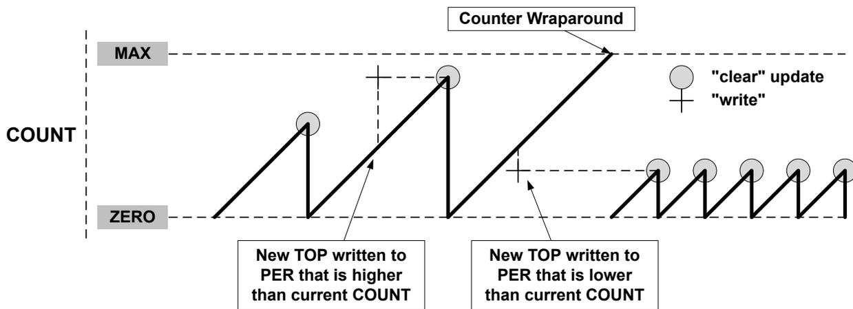
A counter wraparound can occur in any operation mode when up-counting without buffering, see [Figure 35-8](#).
