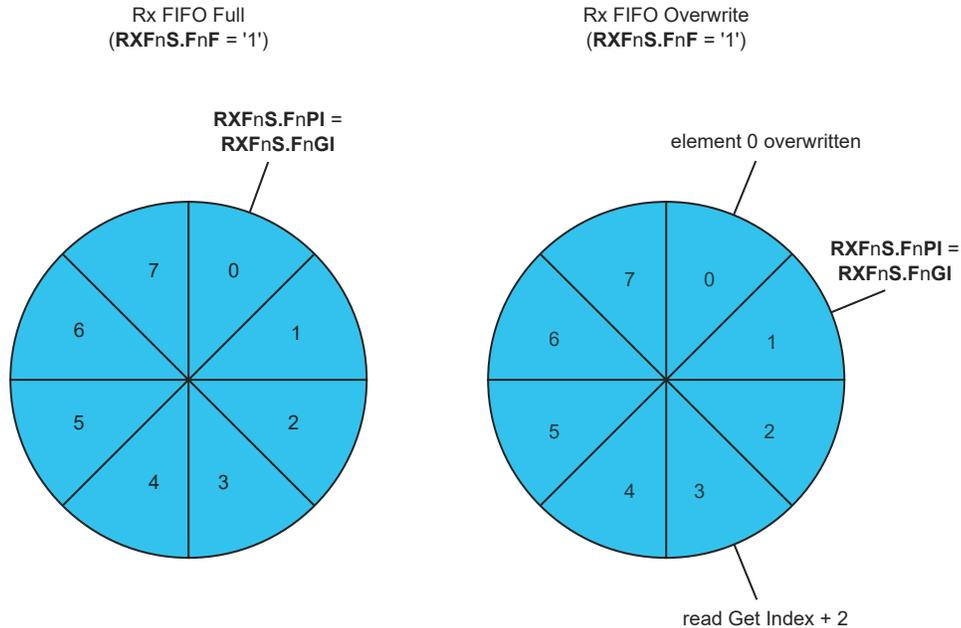
After reading from the Rx FIFO, the number of the last element read has to be written to the Rx FIFO Acknowledge Index RXFnA.FnA. This increments the get index to that element number. In case the put index has not been incremented to this Rx FIFO element, the Rx FIFO full condition is reset (RXFnS.FnF = '0').
