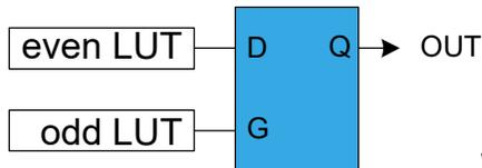
When the even LUT is disabled (LUTCTRL0.ENABLE=0 / LUTCTRL2.ENABLE=0), the latch output will be cleared. The G-input is forced enabled for one more APB clock cycle, and the D-input to zero. In all other cases, the latch output (OUT) is refreshed as shown in [Table 37-4](#).
