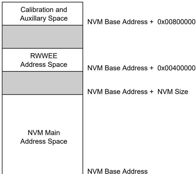
The lower rows in the NVM main address space can be allocated as a boot loader section by using the NVM User Row BOOTPROT fuses, and the upper rows can be allocated to EEPROM Emulation section by using the NVM User Row EEPROM Size fuses, as shown in the figure below.
