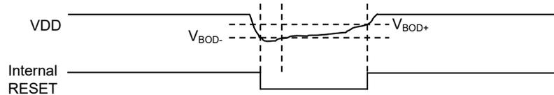
Enabling the BODVDD hysteresis by writing the Hysteresis bit in the BODVDD register (BODVDD.HYST) to '1' will add hysteresis to the BODVDD threshold level.
