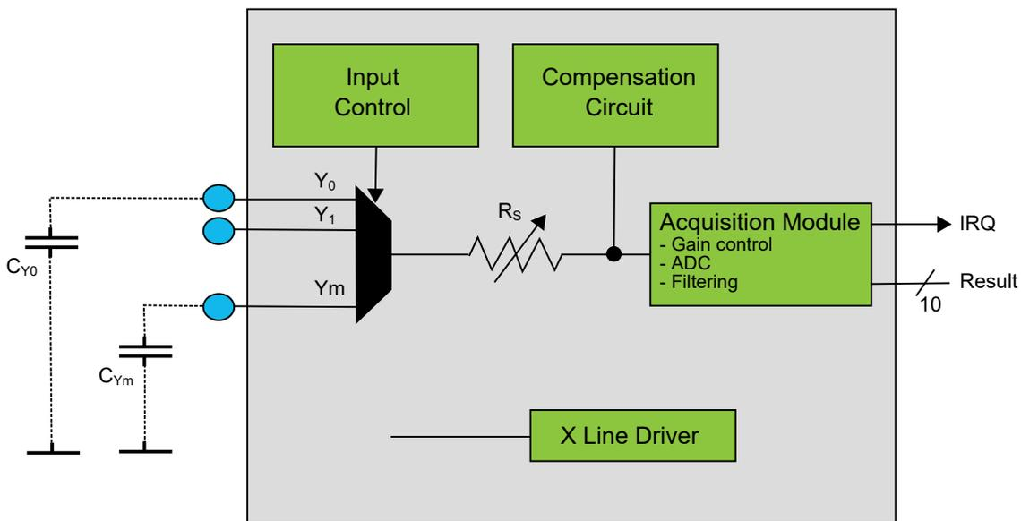
**Note:** For SAM C20/C21 the  $R_s = 0, 20, 50, 100 \text{ K}\Omega$ .
