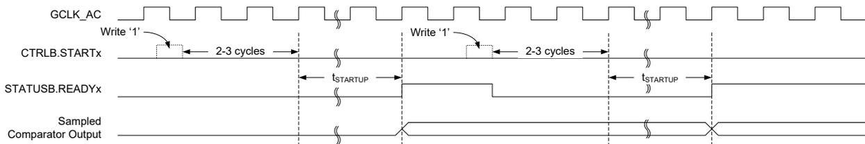
For low-power operation, event-triggered measurements can be performed during sleep modes. When the event occurs, the Power Manager will start GCLK\_AC. The comparator is enabled, and after the startup time has passed, a comparison is done and appropriate peripheral events and interrupts are also generated. The comparator and GCLK\_AC are then disabled again automatically, unless configured to wake up the system from sleep.
