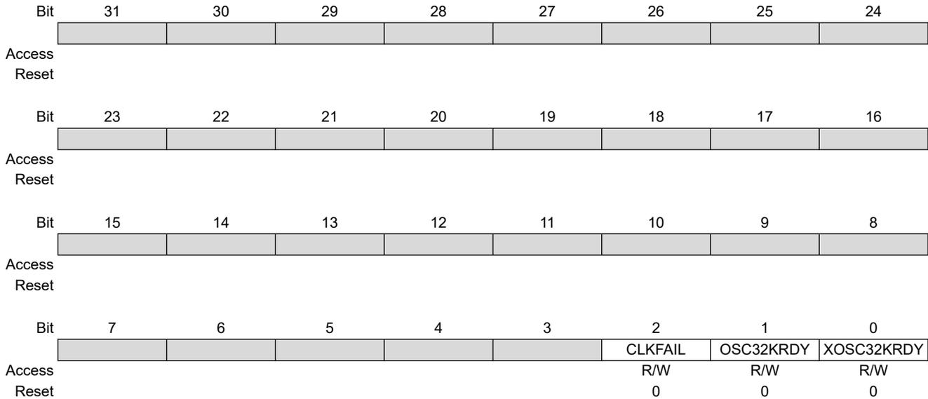
**Bit 2 – CLKFAIL** XOSC32K Clock Failure Detection
