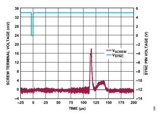
Figure 5. Screw Terminal Voltage ( $V_{SCREW}$ ) and  $\overline{SYNC}$  Pin Voltage ( $\overline{V_{SYNC}}$ ) vs. Time on Voltage Output Enabled
