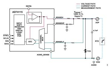
Figure 35. Resistance Measurement Configuration
