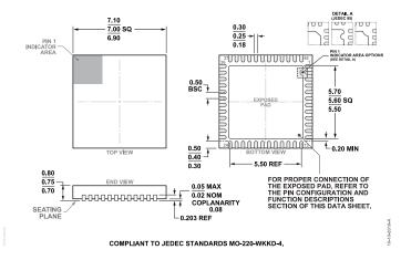
Figure 59. 48-Lead Lead Frame Chip Scale Package [LFCSP] 7 mm × 7 mm and 0.75 mm Package Height (CP-48-13) Dimensions shown in millimeters
