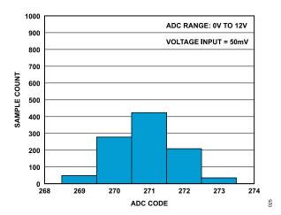
Figure 24. ADC Noise Histogram with ODR = 9.6 kSPS
