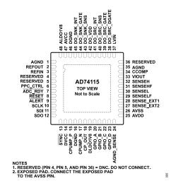
Figure 4. Pin Configuration
