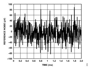
Figure 19. Peak-to-Peak Noise (100 kHz Bandwidth)
