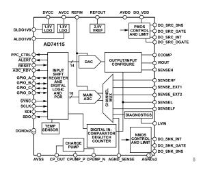
Figure 1. Functional Block Diagram
