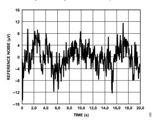
Figure 18. Peak-to-Peak Noise (0.1 Hz to 10 Hz Bandwidth)
