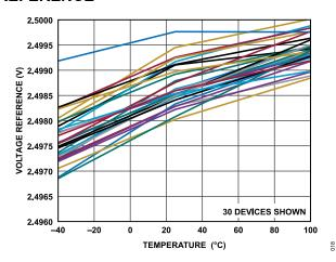
Figure 17. Voltage Reference vs. Temperature
