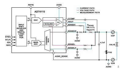
Figure 29. Voltage Output Mode Configuration
