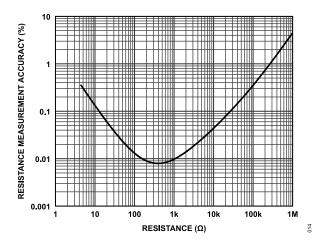
Figure 13. 2-Wire Resistance Measurement Accuracy
