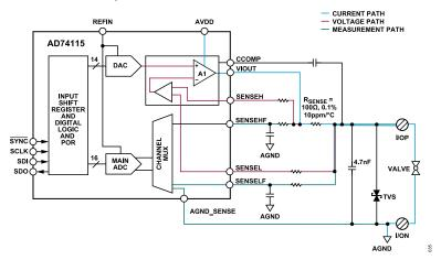
Figure 30. Current Output Mode Configuration
