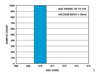
Figure 21. ADC Noise Histogram with ODR = 20 SPS
