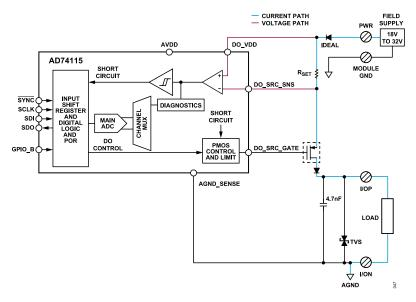
Figure 42. Digital Outputs Sourcing with External FET
