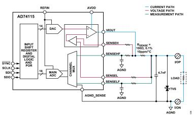
Figure 33. Current Input, Loop Powered Mode Configuration
