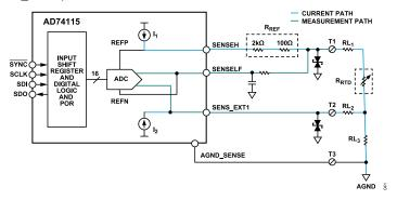
Figure 36. 3-Wire RTD Measurement Configuration
