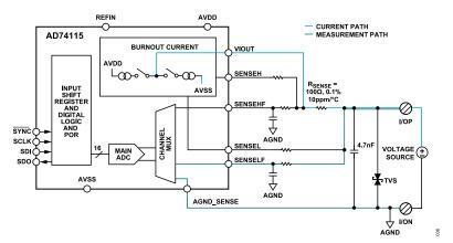
Figure 31. Voltage Input Mode Configuration
