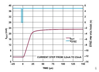
Figure 10.  $I_{OUT}$  and  $\overline{SYNC}$  Pin Voltage ( $V_{\overline{SYNC}}$ ) vs. Time
