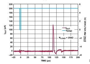
Figure 9. I<sub>OUT</sub> and SYNC Pin Voltage (V<sub>SYNC</sub>) vs. Time on Current Output
