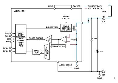
Figure 46. Digital Output Sinking Mode with the Internal FET
