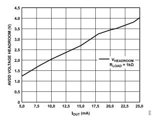
Figure 12. AVDD Voltage Headroom vs. I<sub>OUT</sub>
