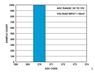
Figure 20. ADC Noise Histogram with Output Data Rate (ODR) = 10 SPS
