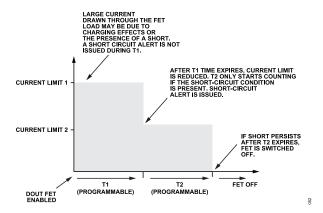
Figure 47. Digital Output Programmable Short-Circuit Control
