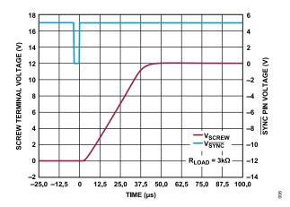
Figure 7. Full-Scale Positive Step Without C<sub>COMP</sub>
