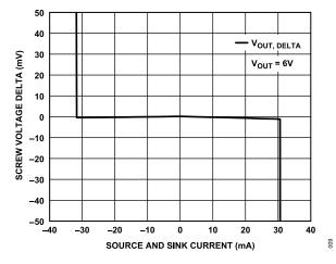
Figure 8. Output Voltage Change ( $V_{\text{OUT, DELTA}}$ ) vs. Source and Sink Current
