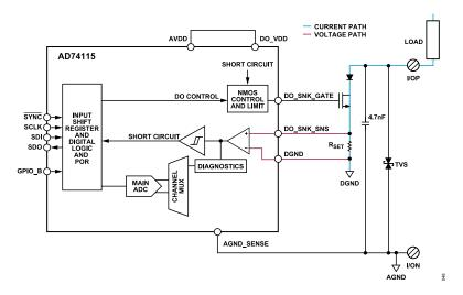
Figure 43. Digital Output Sinking with External FET
