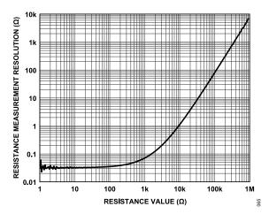
Figure 14. Resistance Measurement Resolution vs. Resistance Value
