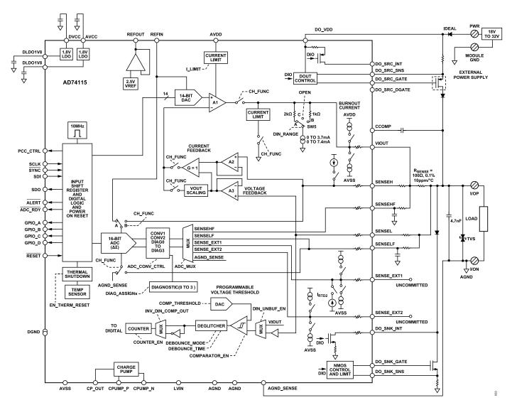
Figure 28. Detailed Functional Block Diagram
