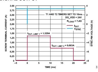
Figure 25. Digital Output Programmable Short-Circuit Activation
