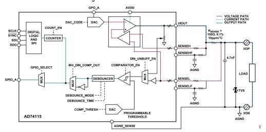
Figure 41. Digital Input, Loop Powered Configuration Mode
