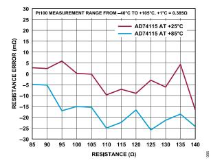
Figure 15. 3-Wire RTD Measurement Error
