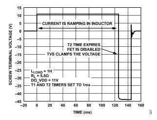
Figure 26. Demagnetization Strategy for Inductive Loads ( $L_{LOAD}$ )
