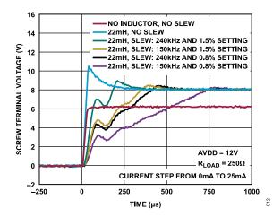
Figure 11. I<sub>OUT</sub> Settling Time with Inductive Load and with and Without Slew Rate Enabled
