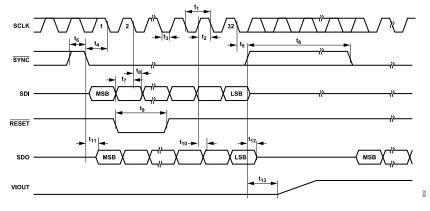
Figure 2. SPI Timing Diagram
