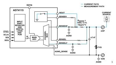
Figure 32. Current Input, Externally Powered Mode Configuration
