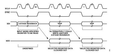
Figure 54. 2-Stage Readback Timing Diagram
