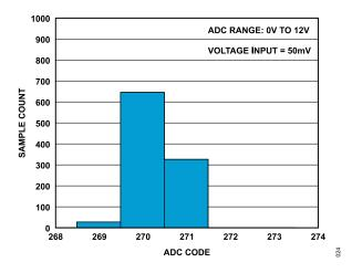
Figure 23. ADC Noise Histogram with ODR = 4.8 kSPS
