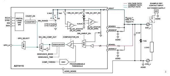
Figure 38. Digital Input Logic Mode Configuration
