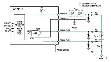
Figure 37. 4-Wire RTD Measurement Configuration
