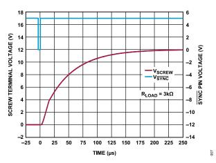
Figure 6. Full-Scale Positive Step with C<sub>COMP</sub> Connected
