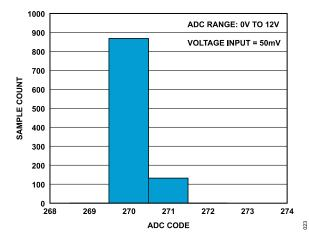
Figure 22. ADC Noise Histogram with ODR = 1.2 kSPS
