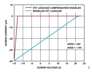
Figure 27. Function of Current Leakage Compensation
