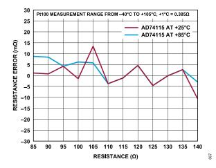
Figure 16. 4-Wire RTD Measurement Error
