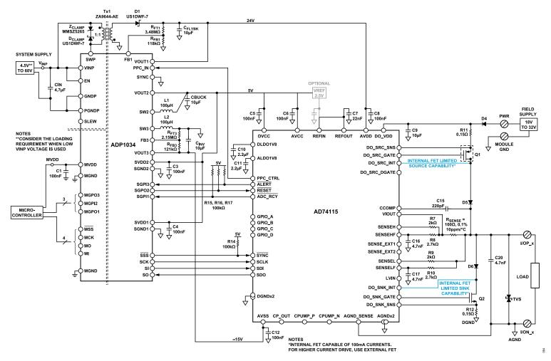
Figure 58. AD74115 and ADP1034 System Level Diagram
