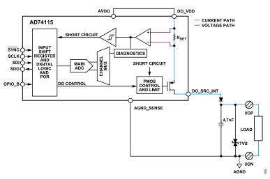
Figure 45. Digital Output Sourcing Mode with the Internal FET
