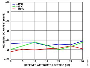
Figure 88. Receiver DC Offset vs. Receiver Attenuator Setting, LO = 1850 MHz
