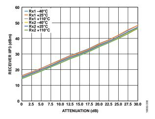
Figure 75. Receiver IIP3 vs. Attenuation, LO = 1800 MHz, Tone 1 = 1802 MHz, Tone 2 = 1892 MHz, -21 dBm Each at Attenuation = 0 dB
