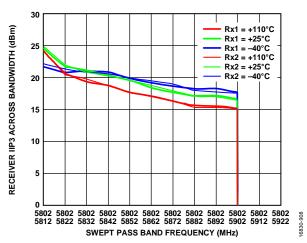
Figure 150. Receiver IIP3 Across Bandwidth vs. Swept Pass Band Frequency, Receiver Attenuation = 0 dB, LO = 5800 MHz, Tone 1 = 5802 MHz, Tone 2 Swept Across Pass Band, -21 dBm Each
