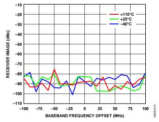
Figure 152. Receiver Image vs. Baseband Frequency Offset, Attenuation = 0 dB, RF Bandwidth = 200 MHz, Tracking Calibration Active,
