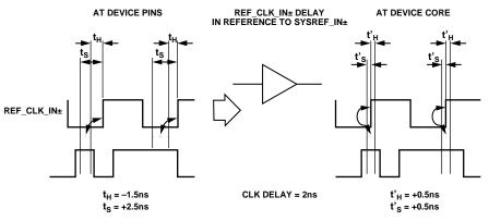
NOTES 1.  $t_{\rm H}$  and  $t_{\rm S}$  are the hold and setup times for the ref\_clk\_in± pins.  $t_{\rm H}'$  and  $t_{\rm S}'$  refer to the delayed hold and setup times at the device core in reference to the sysref\_n± signals due to an internal buffer that the signal passes through.
