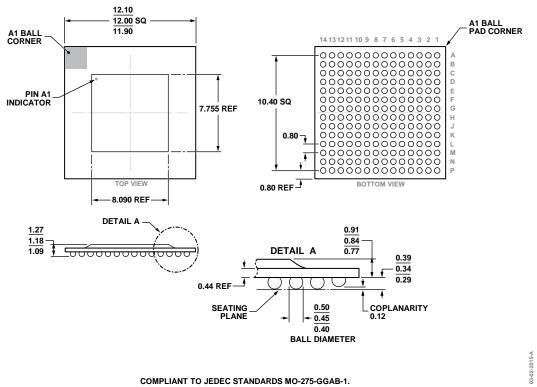
Figure 191. 196-Ball Chip Scale Package Ball Grid Array [CSP\_BGA] (BC-196-13) Dimensions shown in millimeters
