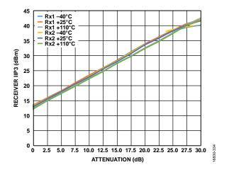
Figure 71. Receiver IIP3 vs. Attenuation, LO = 1800 MHz, Tone 1 = 1890 MHz, Tone 2 = 1891 MHz, -21 dBm Each at Attenuation = 0 dB
