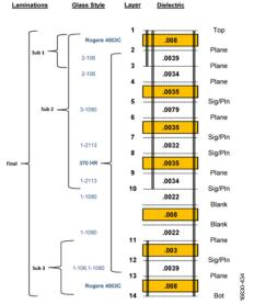
Figure 170. ADRV9008-1W/PCBZ Trace Impedance and Stackup
