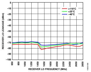
Figure 54. Receiver LO Leakage vs. Receiver LO Frequency, Receiver Attenuation = 0 dB, RF Bandwidth = 200 MHz, Sample Rate = 245.76 MSPS
