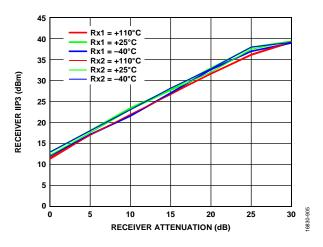
Figure 147. Receiver IIP3 vs. Receiver Attenuation, LO = 5800 MHz, Tone 1 = 5895 MHz, Tone 2 = 5896 MHz, -21 dBm Plus Attenuation
