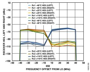
Figure 92. Receiver HD3, Left and Right vs. Frequency Offset from LO, Tone Level = -15 dBm at Attenuation = 0 dB, LO = 650 MHz
