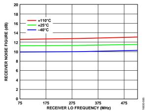
Figure 10. Receiver Noise Figure vs. Receiver LO Frequency, Receiver Attenuation = 0 dB, RF Bandwidth = 50 MHz, Sample Rate = 61.44 MSPS, Integration Bandwidth = ±25 MHz
