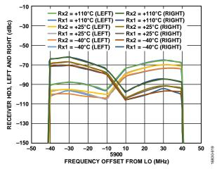
Figure 162. Receiver HD3, Left and Right vs. Frequency Offset from LO, Tone Level = -15 dBm at Attenuation = 0 dB, LO = 5900 MHz
