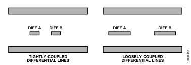
Figure 179. Routing JESD204B, Diff A and Diff B Correspond to Differential Positive Signals or Negative Signals (One Differential Pair)
