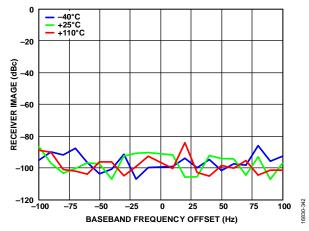
Figure 79. Receiver Image vs. Baseband Frequency Offset, Attenuation = 0 dB, 200 MHz RF Bandwidth, Tracking Calibration Active, Sample Rate = 245.76 MSPS, LO = 650 MHz
