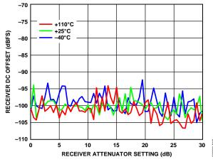
Figure 38. Receiver DC Offset vs. Receiver Attenuator Setting, LO = 75 MHz
