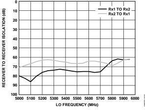
Figure 166. Receiver to Receiver Isolation vs. LO Frequency
