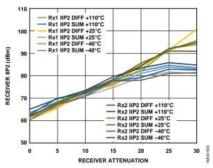
Figure 145. Receiver IIP2 vs. Receiver Attenuation, LO = 5800 MHz, Tones Placed at 5802 MHz and 5892 MHz, -21 dBm Plus Attenuation
