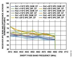
Figure 112. Receiver IIP2 Sum and Difference Across Bandwidth vs. Swept Pass Band Frequency, Receiver Attenuation = 0 dB, LO = 4600 MHz, Tone 1 = 4602 MHz, Tone 2 Swept, -21 dBm Each, IIP2\_SUM\_CF and IIP2\_DIF\_CF Indicate Sum and Difference Products
