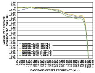
Figure 86. Normalized Receiver Baseband Flatness vs. Baseband Offset Frequency, LO = 2600 MHz
