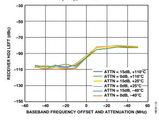
Figure 91. Receiver HD2 Left vs. Baseband Frequency Offset and Attenuation, Tone Level = -15 dBm at Attenuation = 0 dB, HD2 Correction Configured for Low-Side Optimization, X-Axis = Baseband Frequency Offset of the Fundamental Tone and Not the Frequency of the HD2 Product (HD2 Product = 2× the Baseband Frequency), LO = 2850 MHz
