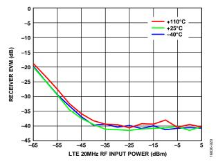
Figure 163. Receiver EVM vs. LTE 20 MHz RF Input Power, LTE 20 MHz RF Signal, LO = 5200 MHz, Default AGC Settings
