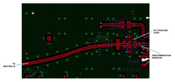
Figure 173. REF\_CLK\_IN± Routing Recommendation
