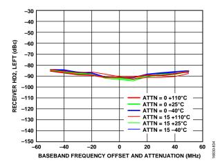
Figure 133. Receiver HD2, Left vs. Baseband Frequency Offset and Attenuation, Tone Level = –15 dBm at Attenuation = 0 dB, X-Axis = Baseband Frequency Offset of the Fundamental Tone Not the Frequency of the HD2 Product (HD2 Product = 2× the Baseband Frequency), HD2
