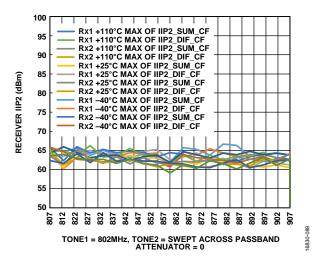
Figure 68. Receiver IIP2 Sum and Difference Across Bandwidth, Receiver Attenuation = 0 dB, LO = 800 MHz, Tone 1 = 802 MHz, Tone 2 Swept, -21 dBm Each, IIP2\_SUM\_CF and IIP2\_DIF\_CF Indicate Sum and Difference Products
