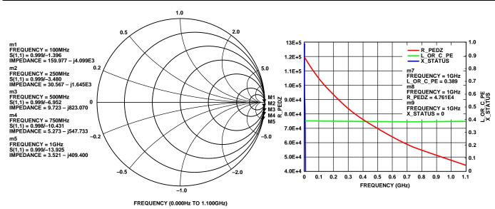
Figure 185. REF\_CLK\_IN $\pm$  SEDZ and PEDZ Data—On Average, the Real Part of Parallel Equivalent Differential Impedance ( $R_P$ ) =  $\sim$ 70 k $\Omega$
