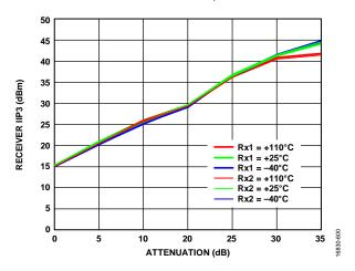
Figure 22. Receiver IIP3 vs. Attenuation, LO = 300 MHz, Tone 1 = 302 MHz, Tone 2 = 322 MHz, -19 dBm Plus Attenuation
