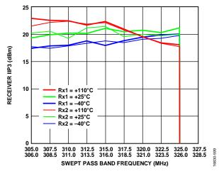
Figure 21. Receiver IIP3, Receiver Attenuation = 0 dB, LO = 300 MHz, Tone 2 = Tone 1 + 1 MHz, -21 dBm Each, Swept Across Pass Band
