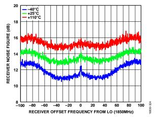
Figure 60. Receiver Noise Figure vs. Receiver Offset Frequency from LO, Integration Bandwidth =  $200\,\text{kHz}$ , LO =  $1850\,\text{MHz}$
