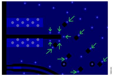
Figure 181. Current Steering Vias Placed Next to Isolation Structures
