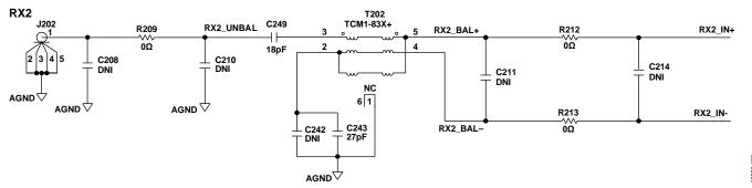
Figure 190. Receiver 1 (RX1) and Receiver 2 (RX2) Generic Matching Network Topology
