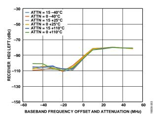
Figure 89. Receiver HD2 Left vs. Baseband Frequency Offset and Attenuation,
