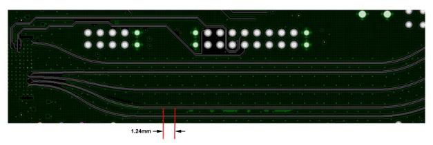
Figure 182. Via Fencing Around JESD204B Lines, PCB Layer 10
