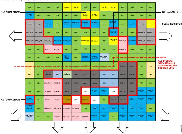
Figure 177. AUXADC\_x, Analog, and Digital GPIO Signals Routing Guidelines
