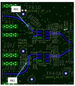
Figure 178. Pi Network Matching Components Available on Different RF Nets
