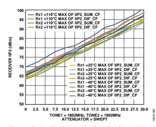
Figure 67. Receiver IIP2, LO = 1800 MHz, Tones Placed at 1802 MHz and 1892 MHz, –21 dBm Each at Attenuation = 0 dB, IIP2\_SUM\_CF and IIP2\_DIF\_CF Indicate Sum and Difference Products
