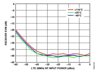
Figure 164. Receiver EVM vs. LTE 20 MHz RF Input Power, LTE 20 MHz RF Signal, LO = 5500 MHz, Default AGC Settings
