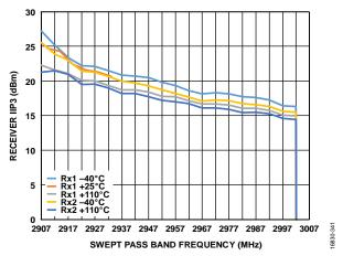
Figure 78. Receiver IIP3 vs. Swept Pass Band Frequency, Receiver Attenuation =  $0 \, dB$ ,  $LO = 2900 \, MHz$ , Tone  $1 = 2902 \, MHz$ , Tone  $2 \, Swept Across Pass Band$ ,  $-21 \, dBm Each$
