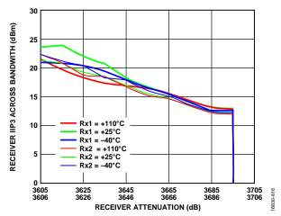
Figure 115. Receiver IIP3 Across Bandwidth, Receiver Attenuation = 0 dB, LO = 3600 MHz, Tone 2 = Tone 1 + 1 MHz, -21 dBm Each,
