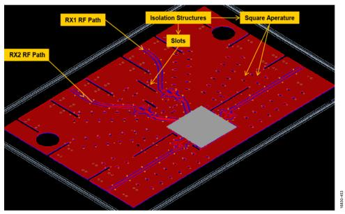
Figure 180. Isolation Structures on the ADRV9008-1W-PCBZ
