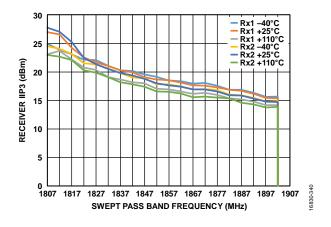
Figure 77. Receiver IIP3 vs. Swept Pass Band Frequency, Receiver Attenuation = 0 dB, LO = 1800 MHz, Tone 1 = 1802 MHz, Tone 2 Swept Across Pass Band, -21 dBm Each
