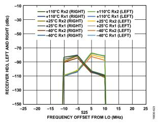
Figure 45. Receiver HD3, Left and Right vs. Frequency Offset from LO, Tone Level – 17 dBm at Attenuation = 0 dB, LO = 525 MHz
