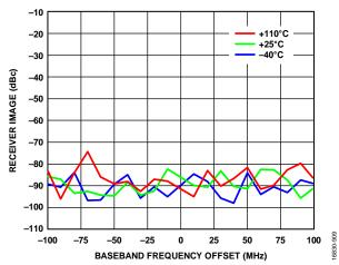
Figure 151. Receiver Image vs. Baseband Frequency Offset, Attenuation = 0 dB, RF Bandwidth = 200 MHz, Tracking Calibration Active, Sample Rate = 245.76 MSPS, LO = 5200 MHz
