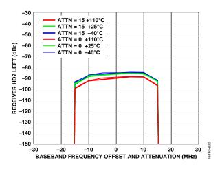
Figure 42. Receiver HD2 Left vs. Baseband Frequency Offset and Attenuation, Tone Level –21 dBm at Attenuation = 0 dB, X-Axis Is Baseband Frequency Offset of Fundamental Tone, Not Frequency of HD2 Product (HD2 Product Is 2×Baseband Frequency), HD2 Canceller Disabled, LO = 525 MHz
