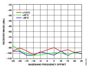
Figure 25. Receiver Image vs. Baseband Frequency Offset, Attenuation = 0 dB, RF Bandwidth = 50 MHz, Tracking Calibration Active, Sample Rate = 61.44 MSPS, LO = 300 MHz
