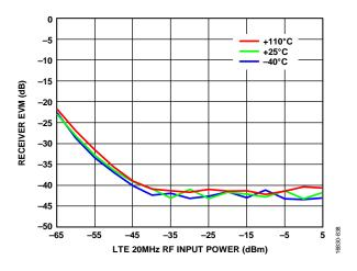
Figure 137. Receiver EVM vs. LTE 20 MHz RF Input Power, RF Signal = LTE 20 MHz, LO = 3600 MHz, Default AGC Settings
