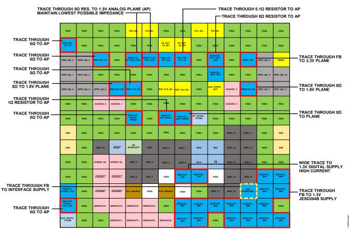
Figure 175. Power Supply Domains Interconnection Guidelines
