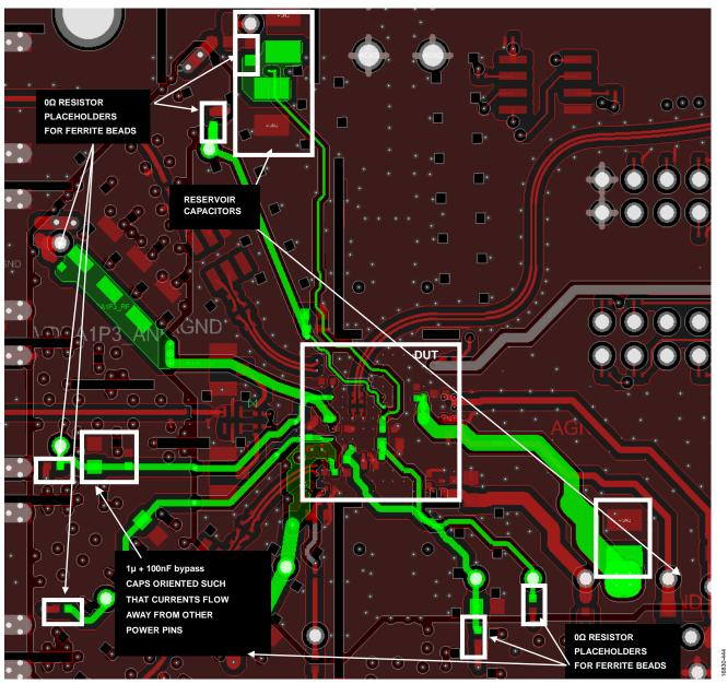
Figure 176. Placement Example of 0  $\Omega$  Resistor Placeholders for Ferrite Beads, Reservoir and Bypass Capacitors on the ADRV9008-1W/PCBZ (Layer 12 to Power and Bottom)
