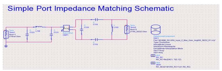
Figure 186 Simulation Setup in ADS with SEDZ **.s1p** Files and DataAccessComponent
