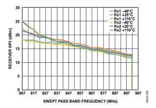
Figure 76. Receiver IIP3 vs. Swept Pass Band Frequency, Receiver Attenuation = 0 dB, LO = 800 MHz, Tone 1 = 802 MHz, Tone 2 Swept Across Pass Band, -21 dBm Each
