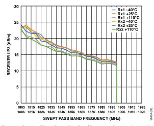
Figure 73. Receiver IIP3 vs. Swept Pass Band Frequency, Receiver Attenuation = 0 dB, LO = 1800 MHz, Tone 2 = Tone 1 + 1 MHz, -21 dBm Each,
