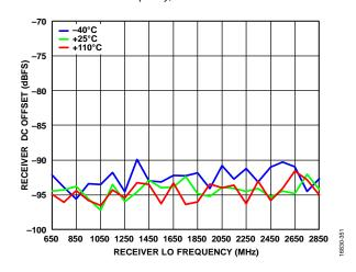
Figure 87. Receiver DC Offset vs. Receiver LO Frequency
