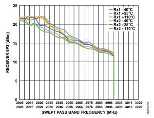
Figure 74. Receiver IIP3 vs. Swept Pass Band Frequency, Receiver Attenuation = 0 dB, LO = 2900 MHz, Tone 2 = Tone 1 + 1 MHz, -21 dBm Each,
