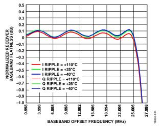
Figure 36. Normalized Receiver Baseband Flatness vs. Baseband Offset Frequency (Receiver Flatness), LO = 75 MHz
