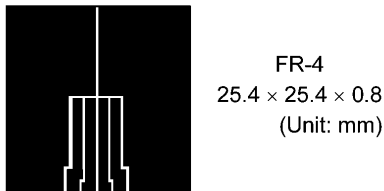
Fig. 5.1 Device Mounted on a Glass-Epoxy Board (a)
