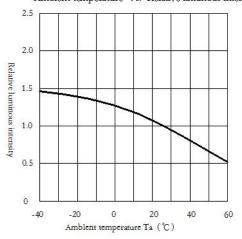
Fig.5 Relative Radiant Intensity
