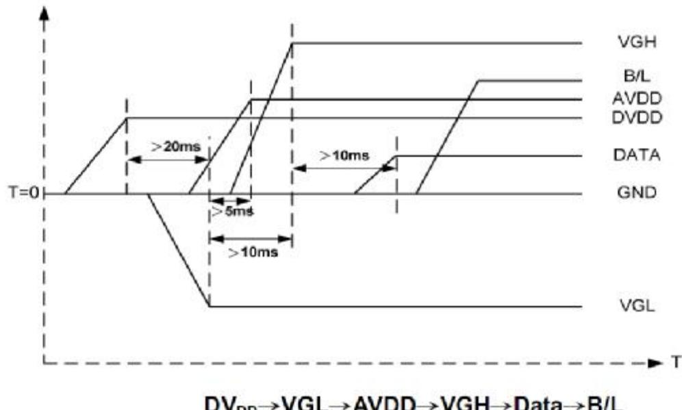
$DV_{DD} \rightarrow VGL \rightarrow AVDD \rightarrow VGH \rightarrow Data \rightarrow B/L$
