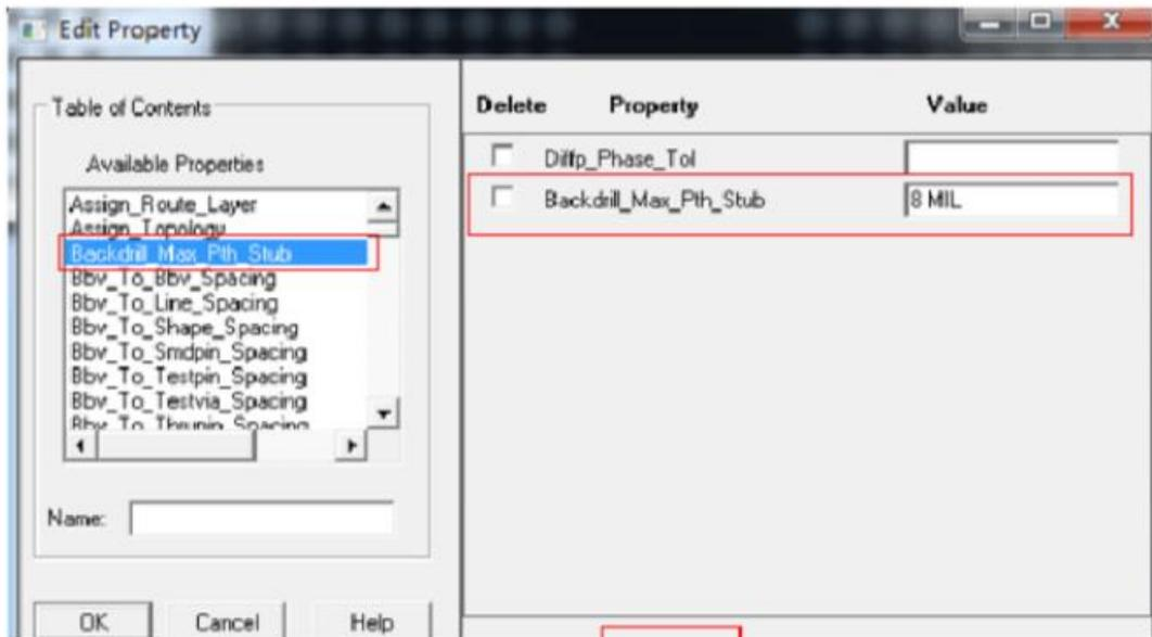
4.选择 Manufacture->NC->Backdrill Setup and Analysis...进入背钻层设置
