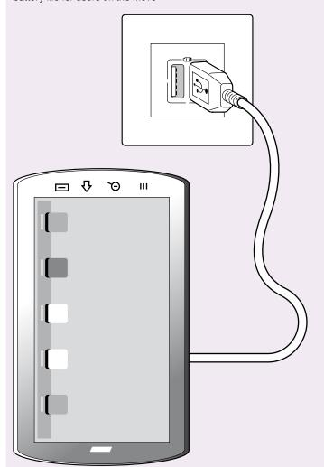
1 500 mA version: can simultaneously charge two mobile terminals conforming to EN 62684 or PC tablet (fast charging)
