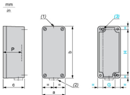
(1) 1 hole, without blanking plug, for cable gland with 14 mm/0.55 in. maximum clamping capacity
